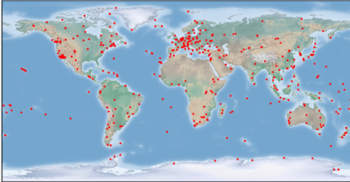
Figure 3: The 507 IGS stations as of January 31, 2019. The IGS collects, archives, and freely distributes Global Navigation Satellite System (GNSS) observation data sets from a cooperatively operated global network of ground tracking stations.
