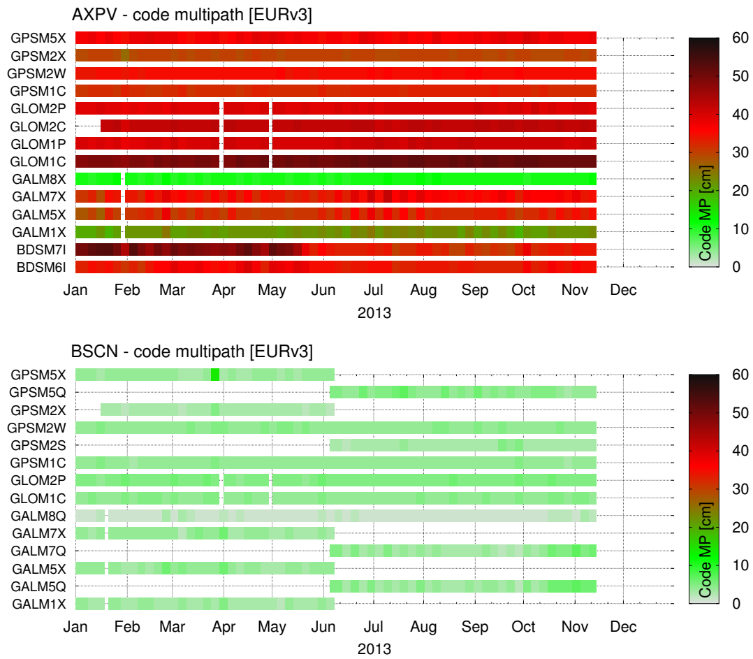
Figure 1: Pseudorange multipath estimated for all GNSS signals observed at the EUREF station AXPV (top) and BSCN (bottom) during January–November, 2013
