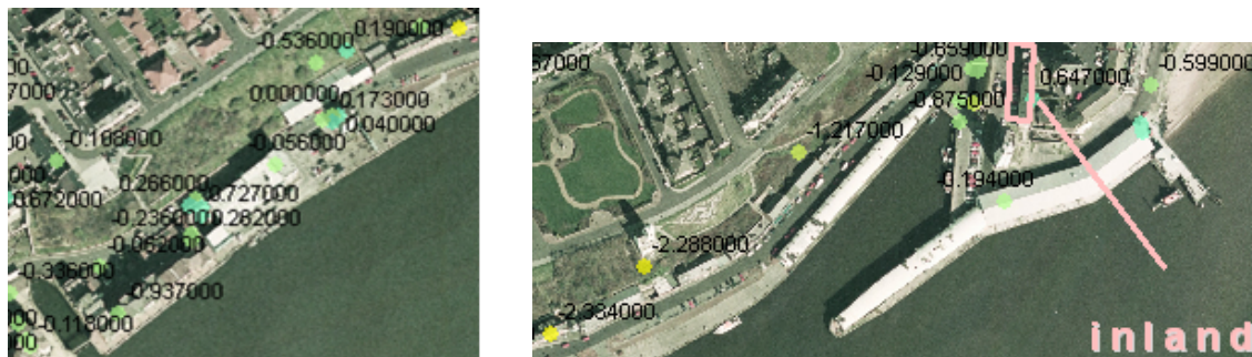
Figure 7: Persistent scatterer points in the areas around the TG (left) and the nearby Lighthouse (right) where the TG benchmarks are located. The PS points indicate that both areas are stable with respect to each other.
