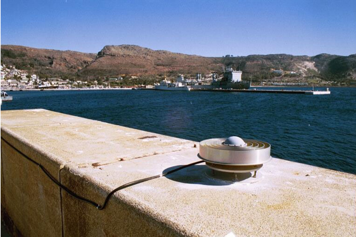
Figure 2. The GPS antenna of SIMO, an IGS TOS station located at Simonstown, South Africa.
