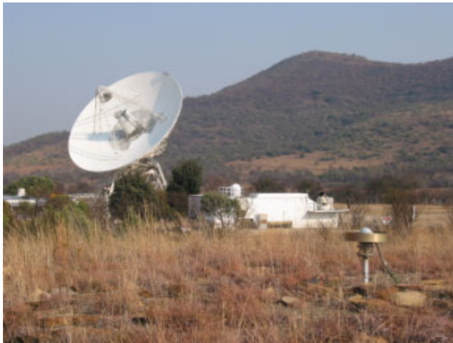
Figure 1. The 26 metre radio telescope used for geodetic VLBI. Solid panels have been fitted as part of a surface upgrade, which is expected to be complete by end 2003. In the foreground is the antenna of the IGS station HRAO and to the right is the NASA SLR MOBLAS6. The collocation of these three geodetic systems makes HartRAO an important contributor to global space geodesy.
