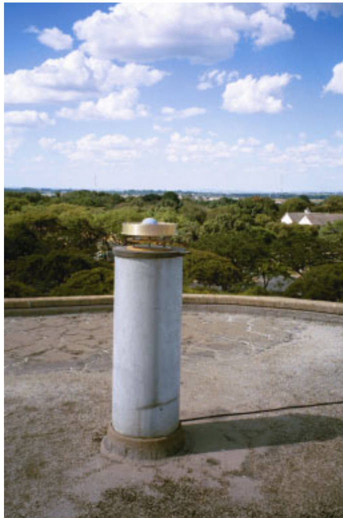
Figure 3. The ZAMB GPS antenna monumentation located in Lusaka, Zambia. The antenna is situated on a massive concrete foundation, which extends through a large building. The foundation used to support a large water tank
