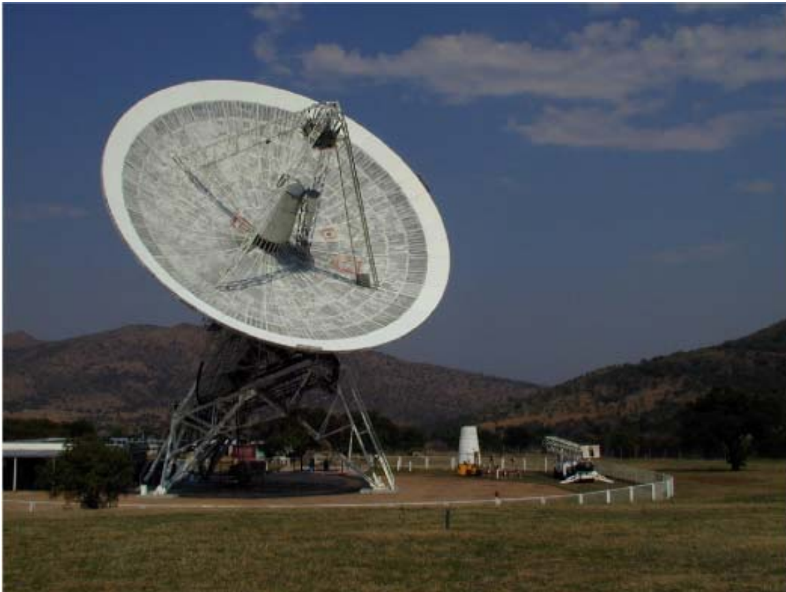
Figure 1. The 26 metre radio telescope. Solid panels have been fitted on the outer ring as part of a surface upgrade. All panels will eventually be replaced with non-perforated, higher tolerance panels. Typical rms accuracy of these panels is 170 microns.
