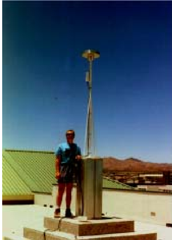
Figure 2. The NAMI GPS antenna monumentation located in Windhoek, Namibia. The antenna needed to be elevated to alleviate the possible adverse effect of multi-pathing from a nearby corrugated iron roof. The pole is thick-walled and stayed for rigidity. NAMI is a regional station at the moment, but it is hoped that an equipment upgrade can bring it to IGS status. (Donors?)
