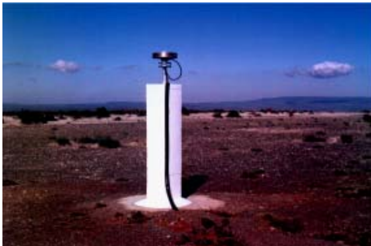
Figure 3. The SUTH IGS GPS antenna monumentation. The antenna is situated on a hill overlooking the barren semi-desert of the Karoo.
