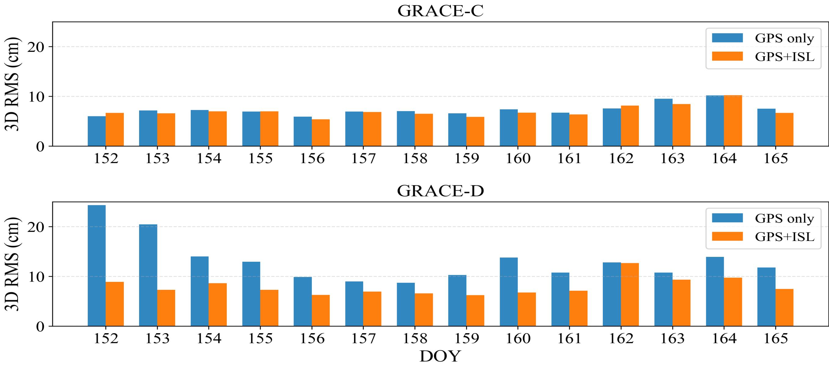
Figure 4. Daily RMS values of orbit errors in the 3D directions obtained using GPS-only and GPS +ISL observations.
