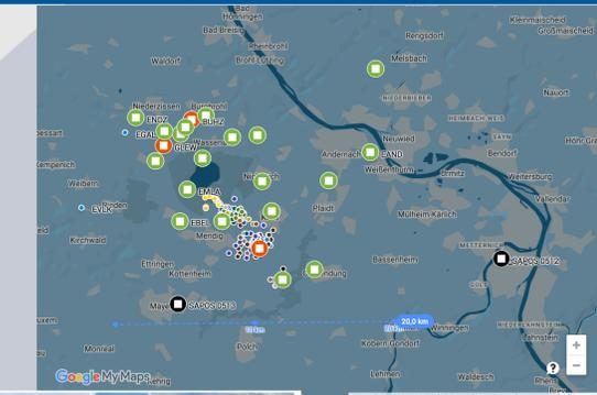
**Fig. 2:** LSV GNSS network: 3 multi-parameter stations as core stations (red), 19 low-cost GNSS stations (green), 2 SAPOS stations (black); smaller dots indicate DLF Earthquakes (the colour indicated depth).
