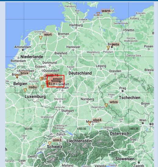
**Fig. 3:** total of 36 stations are included in network processing: 8 IGS stations, 6 Germany SAPOS CORS stations close to Eifel, 22 LSV stations.
