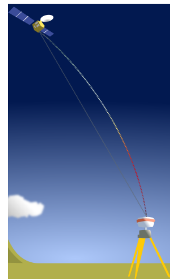
Figure 1. Schematic of the troposphere delay in the GNSS signal propagation.
