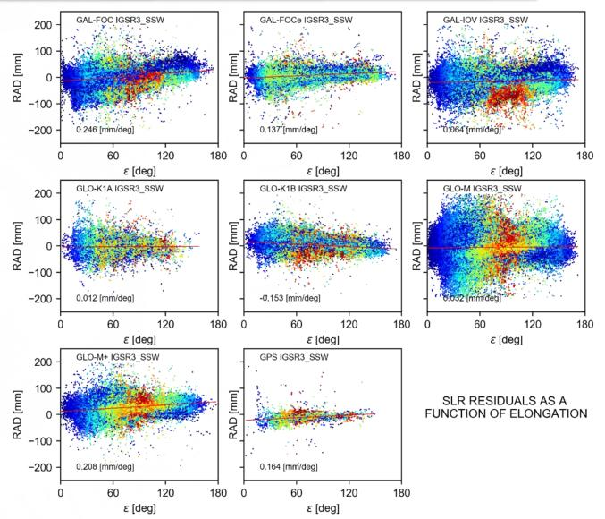
SLR residuals as a function of elongation angle ( $\epsilon$ ). Dots are colored with the absolute height of the Sun above the orbital plane ( $\beta$ )
