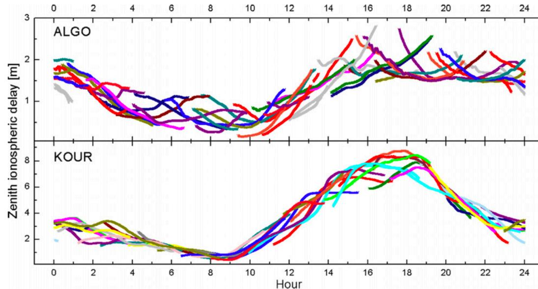
Zenith ionospheric delay which is used as samples for the statistic analysis in the following study. e.g., ALGO (top) and KOUR (bottom) on the DOY 091 2010
