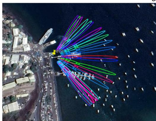
Fig. 2. the screenshot of first Fresnel zones for MAYG, and elevation angles of 5°, 9°, 13°, and 18° projected on a Google Earth image. An  $H_R$  value of 6 m was used.
