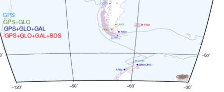
Fig. 3: Present SIRGAS reference frame: it comprises 533 continuously operating GNSS stations: 67 belonging to the IGS global network, 339 tracking GLONASS, 79 tracking GALILEO, and 43 tracking BEIDOU. 122 stations have been decommissioned, but they are included in the SIRGAS reprocessing campaigns.
