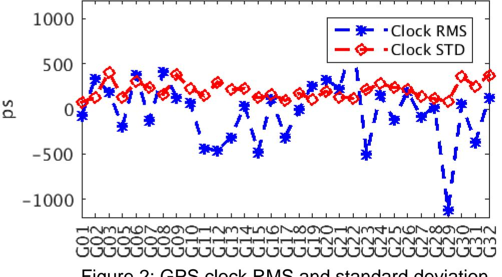
Figure 2: GPS clock RMS and standard deviation
