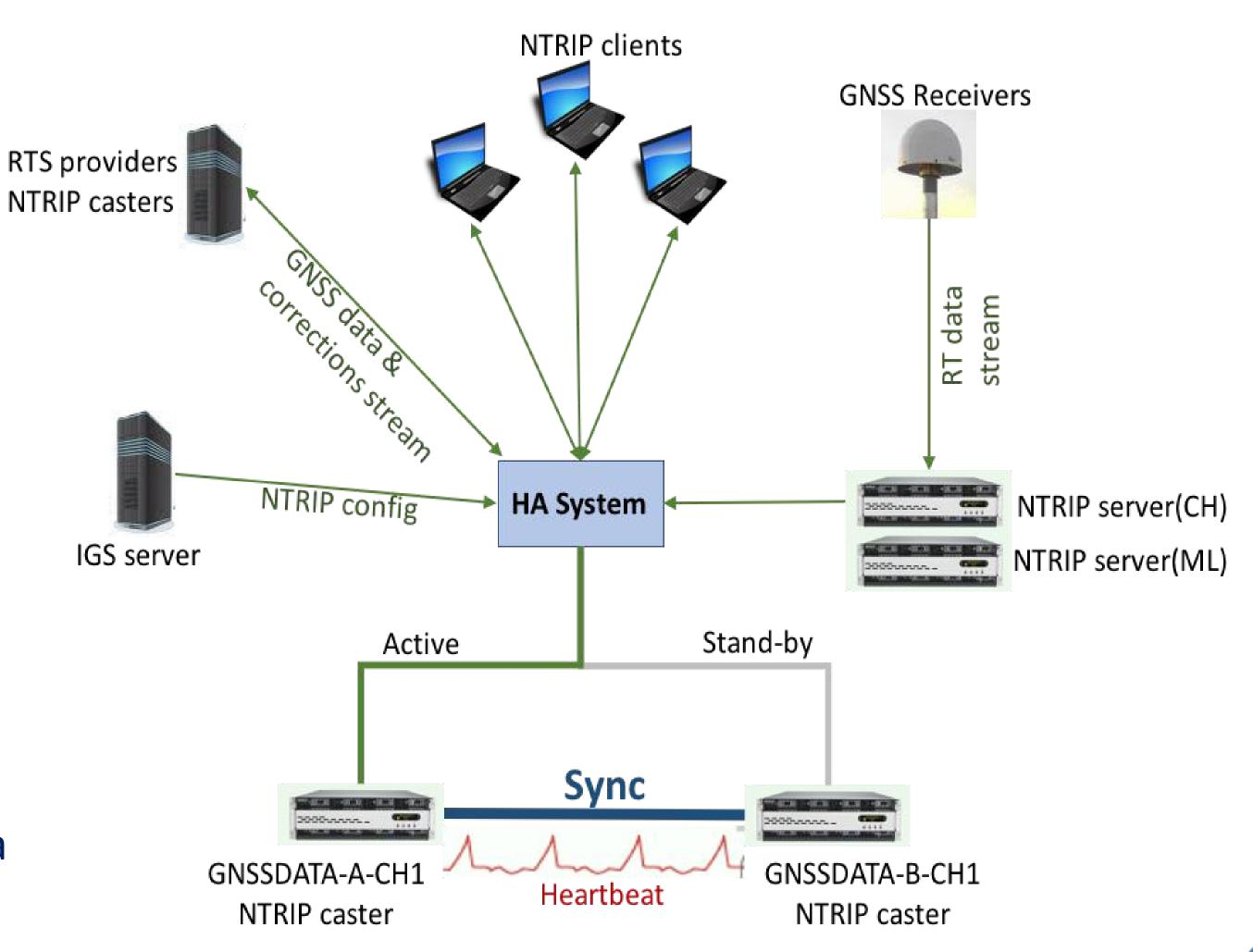
Data synchronization between the main and redundant server is done via Distributed Replicated Block Device (DRBD) device. This enables the stand-by server to be in a safe state and resumes operations without interruption when a switchover occurs.
