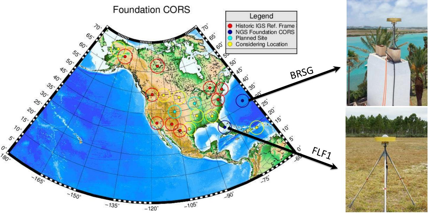
Recently, NGS has installed two pilot stations: one in Bermuda (BRSG) and the other in Miami, Florida (FLF1). NGS' next installation will be at the Table Mountain Gravity Observatory in Boulder, Colorado (nearby TMGO). It will be a Deep-Drilled Braced Monument, and will be co-located with an absolute gravimeter.
