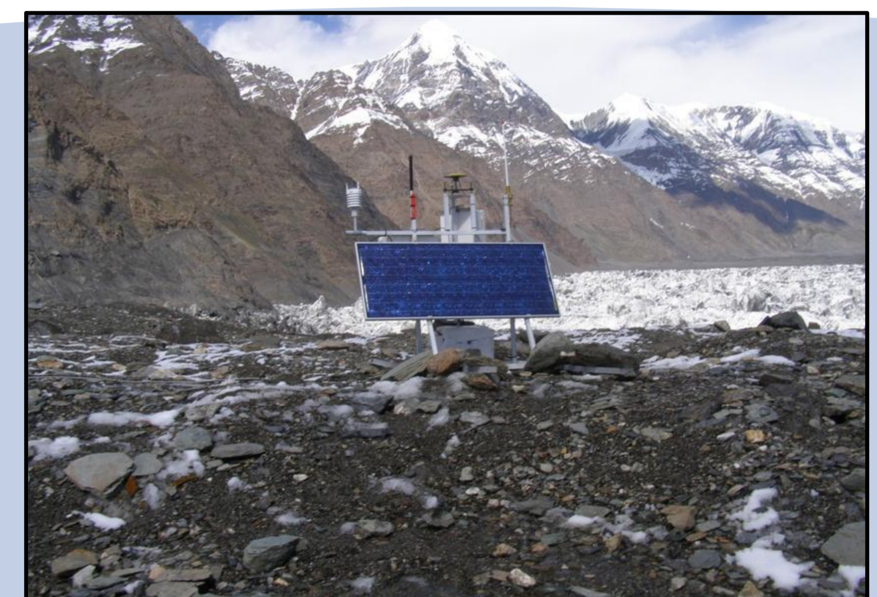
Kinematic ice dam station (ICED) with a Topcon GNSS receiver, a Vaisala WXT520 weather sensor, power supply and HF radio antennas.
