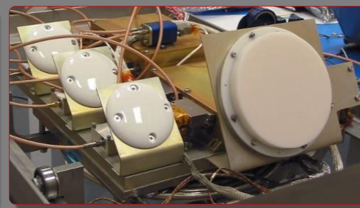
Figure 3: CASSIOPE's GAP GPS antennas under test prior to final installation on the satellite.
