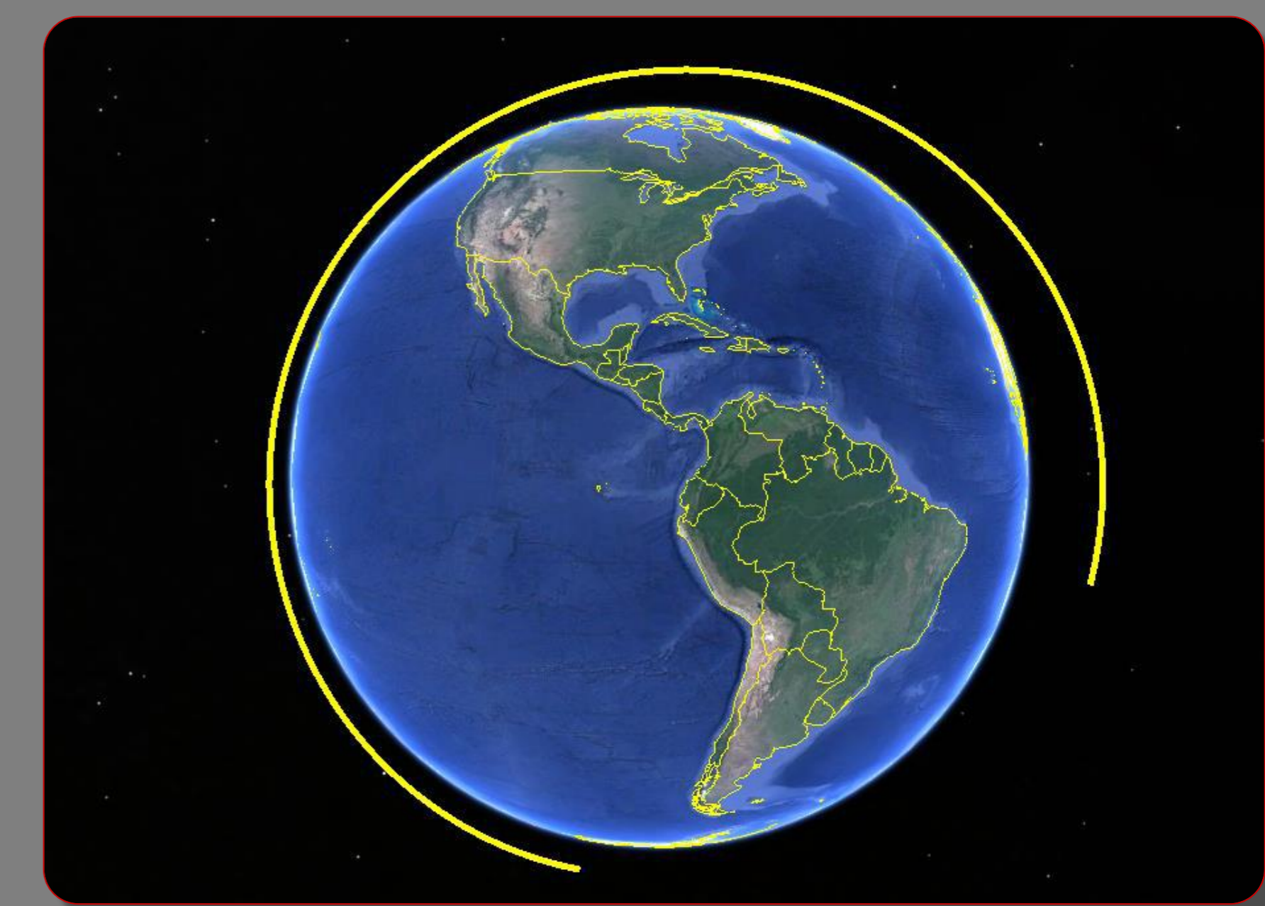
Figure 7: Estimated orbital positions of the CASSIOPE spacecraft via GPS observations from GAP-A receiver 1 on May 5, 2017.
