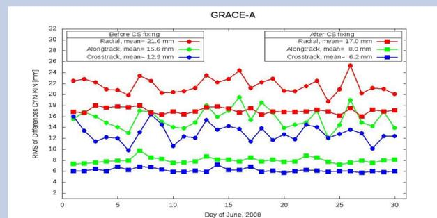
**Fig. 9.** GRACE-A differences between dynamic and kinematic orbits before and after CS fixing. Improvement are mostly pronounced in along- and cross-track direction.
