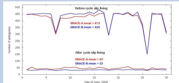
**Fig. 6.** Number of ambiguities before and after CS fixing.
