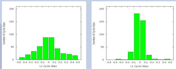
**Fig. 1.** TDX CS distribution for the orbit before (left) and after (right) CS fixing
