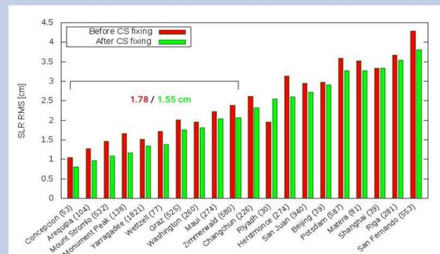
**Fig. 8.** GRACE-A+B SLR statistics for June, 2008. Number of obs. is given in (). Average values are computed from indicated subset of stations.
