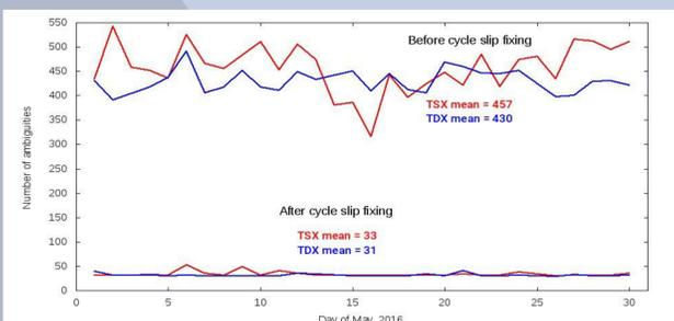
**Fig. 2.** Number of ambiguities before and after the CS fixing.
