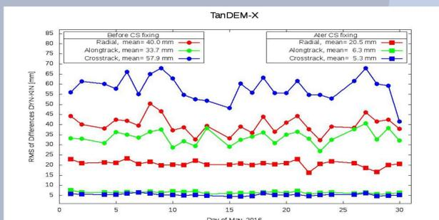
**Fig. 5.** TDX differences between dynamic and kinematic orbits before and after CS fixing. Improvement are mostly pronounced in along- and cross-track direction.
