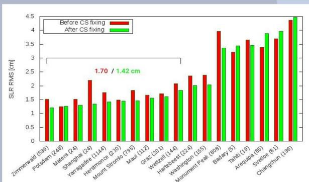
**Fig. 4.** TSX+TDX SLR statistics for May, 2016. Number of observations is given in (). Average values are computed from indicated subset of stations.
