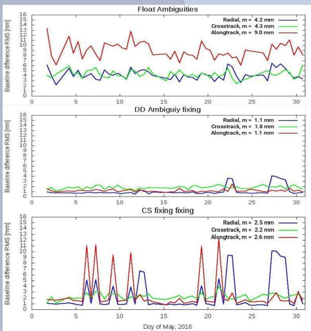
**Fig. 3.** Baseline comparison with precise GFZ baseline solutions. Large deviations are likely caused by smaller number or incorrectly fixed CSs.
