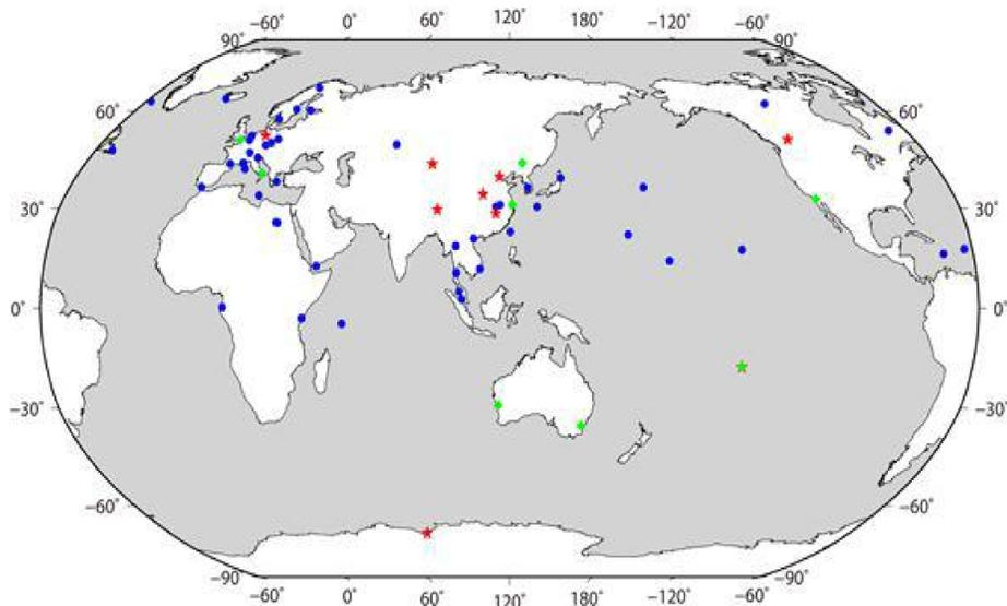
Fig. 1 Tracking stations in precise-orbit determination and satellite laser ranging (SLR) validation for BeiDou-2 and BeiDou-3 satellites. The stations are represented by red five-pointed stars, blue circles, and green diamonds for iGMAS, Multi-GNSS Experiment (MGEX), and SLR stations, respectively.
