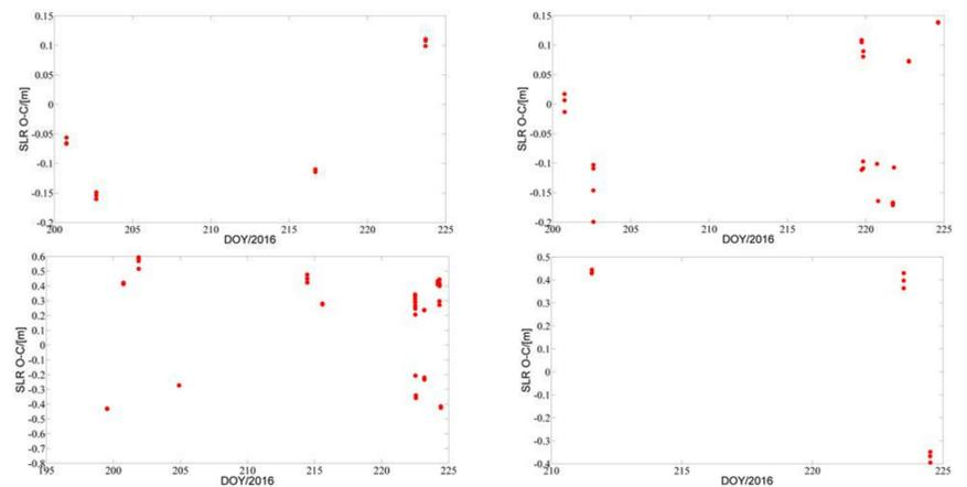
Fig. 6-9 SLR Validation for BeiDou-3 C31, C32, C33, C34 satellites
