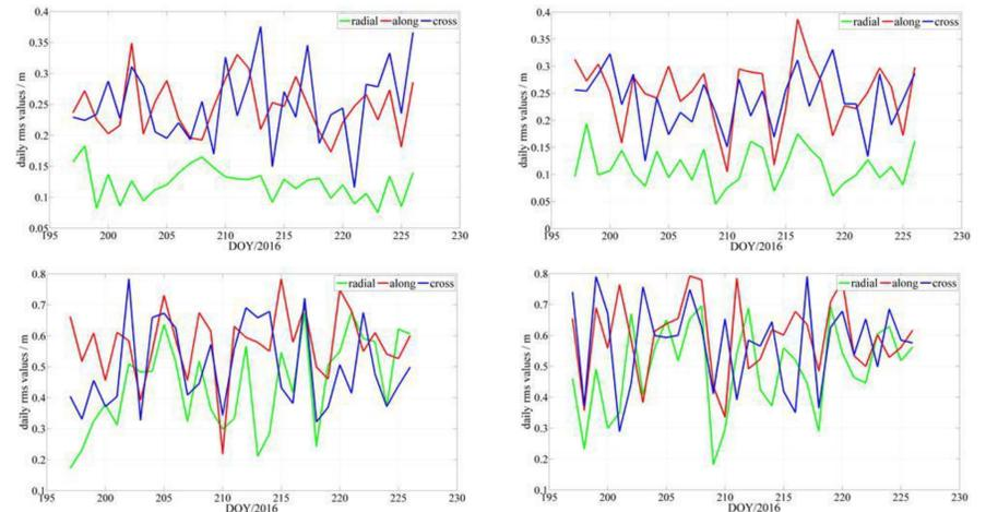
Fig. 2-5 overlap comparison in the radial, along, and cross-track components for BeiDou-3 C31, C32, C33, C34 satellites
