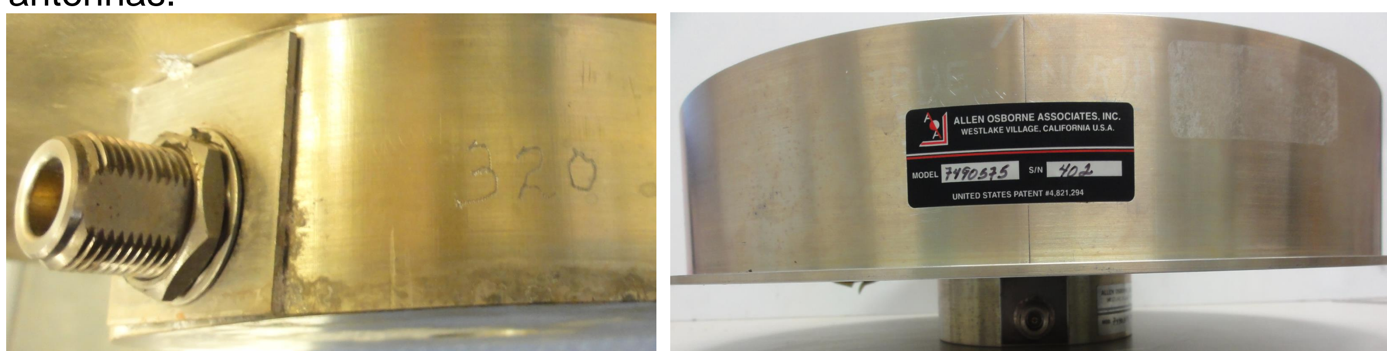
Figure #2: Different styles of serial number marking on AOAD/M_T antennas
