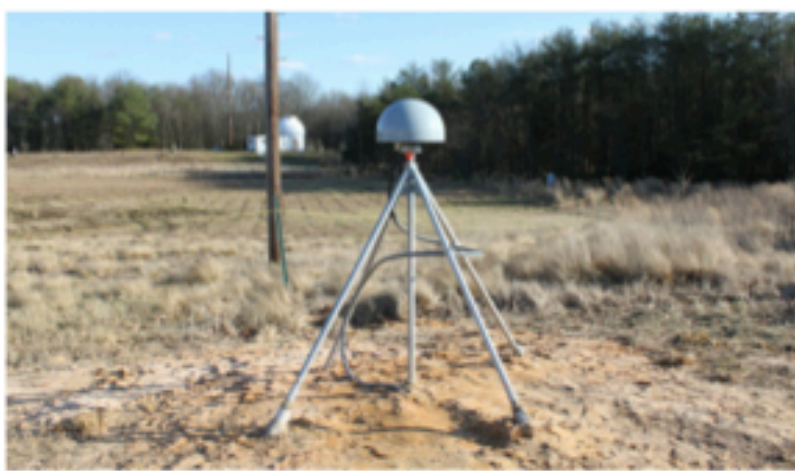
(Left) GODS GNSS south site with deep drilled-braced monument.
