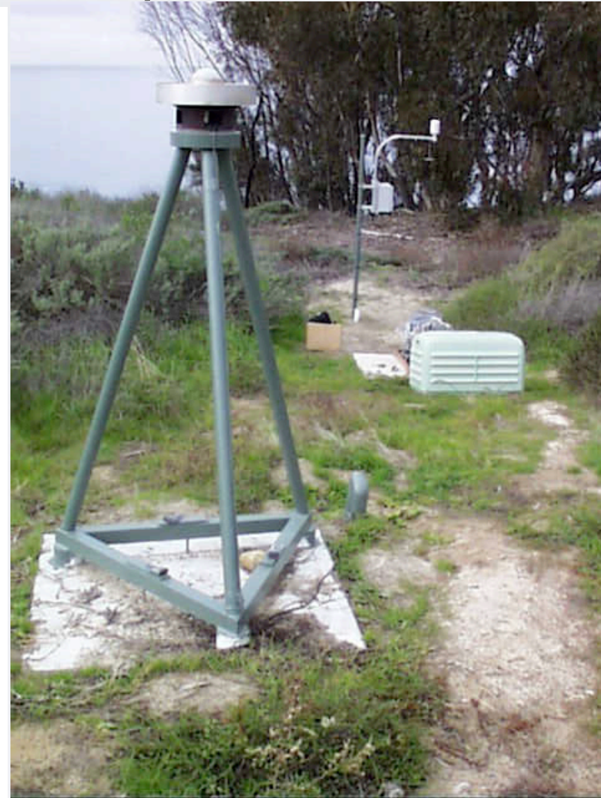
Figure 2. Permanent GPS sites. The heavy lines show the monument, constructed of stainless steel rod. Each of the four legs extends 6 to 8 m into the ground. A pipe (shaded) encloses the monument. The pipe is in a hole of one cubic yard, and concrete fills the space between the pipe and the sides of the hole.
