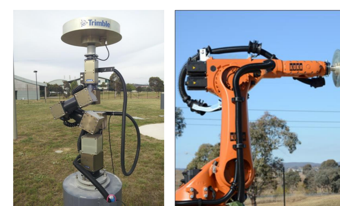
Figure 6: GNSS antenna calibration facility at Geoscience Australia.
