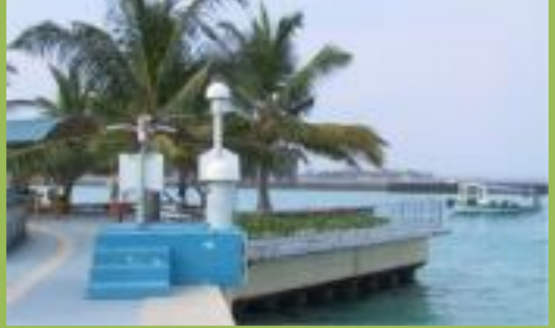
GPS antenna on tide gauge station in Male (Maldives)
