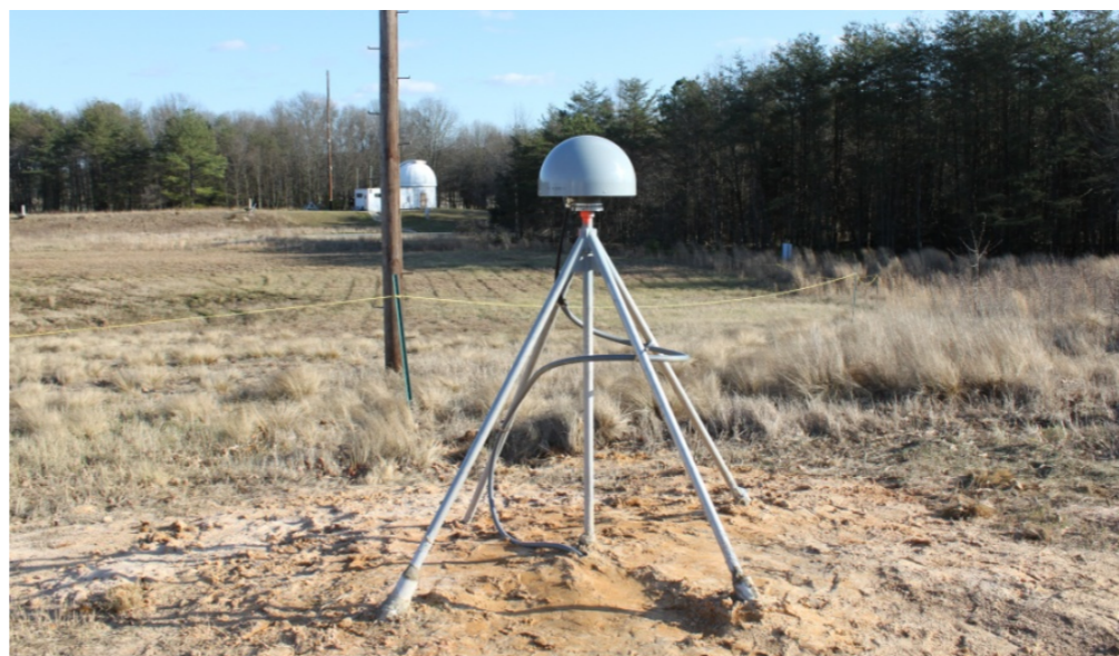
(Left) GODS GNSS south site with deep drilled-braced monument.
