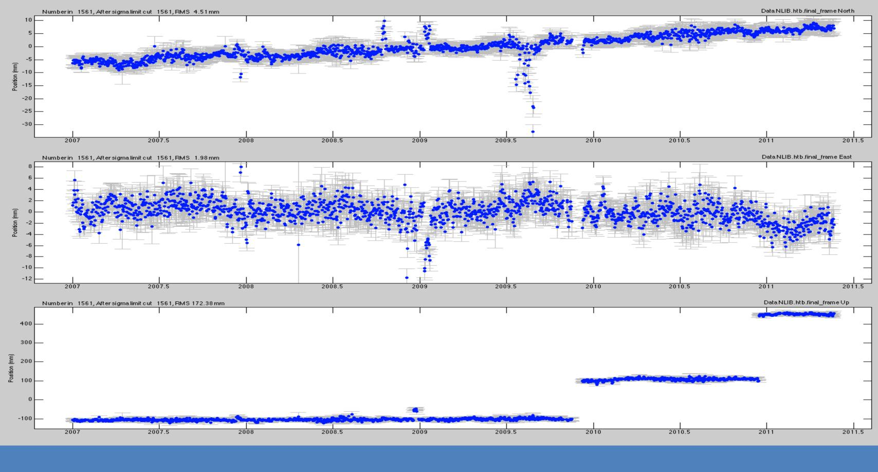
Changes at these stations require precise and delicate modification in order to adequately account for position offsets due to such equipment upgrades. UNAVCO and JPL have collaborated in the design and development of a new set of monument hardware. NASA's Space Geodesy Project
