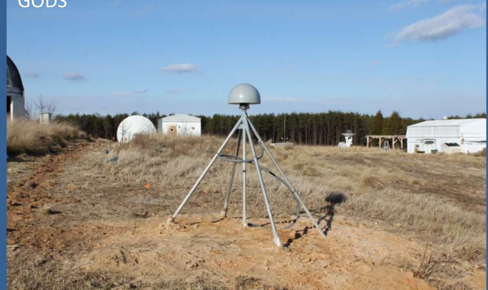
UNAVCO in collaboration with JPL recently installed two deep drilled-braced monuments at the Goddard Geophysical and Astronomical Observatory in early January. These monuments, operating with multi-constellation capable receivers and using calibrated antenna/radome pairs, are part of NASA's Space Geodesy Project, a joint effort led by Goddard Space Flight Center and Jet Propulsion Laboratory. The project is focused on developing, constructing,
