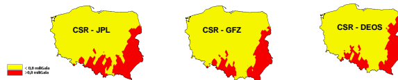
Fig. 3. Differences between gravity anomalies counted on a basis of GRACE data from different calculating centers on the territory of Poland, in red – difference higher than 0,8 milIGala
