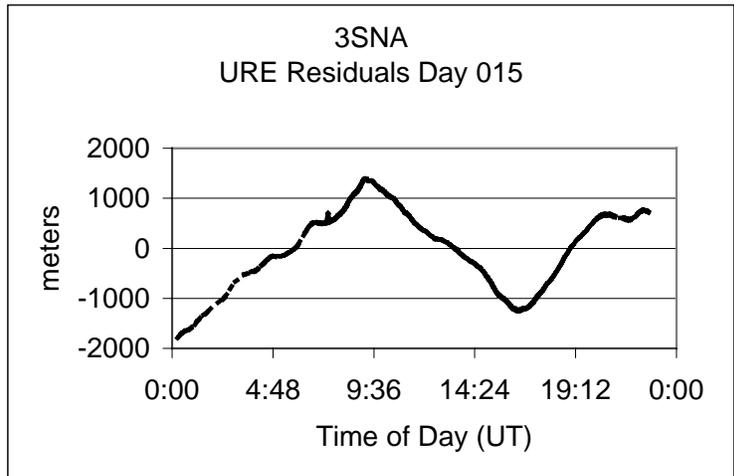
**Figure 5.** Site 3SNA URE residual errors for day 015 (Jan. 15, 1999). The analysis software produces the large errors because the clock behavior is not properly modeled.
