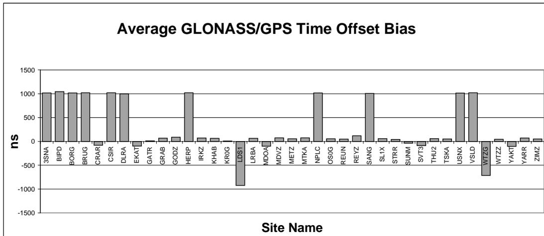
**Figure 1.** This figure shows the average of the daily GLONASS/GPS time offset bias for each site. The sites are listed alphabetically.
