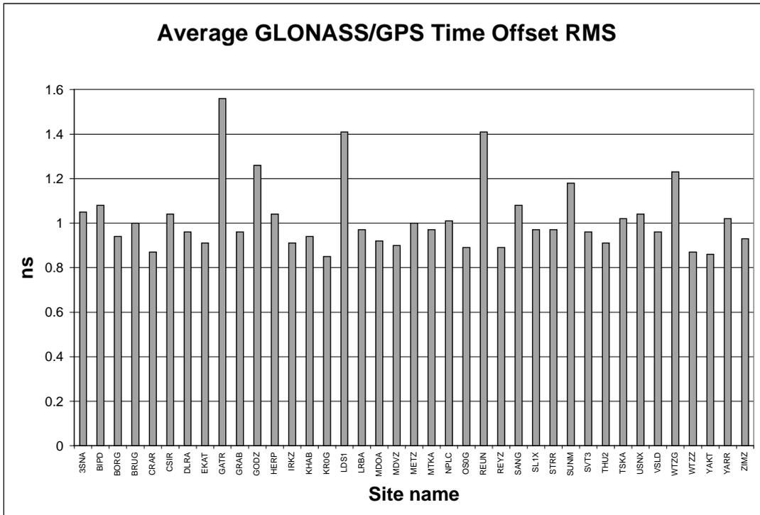
**Figure 2.** This figure shows the average of the daily GLONASS/GPS time offset rms for each site. The sites are listed alphabetically.
