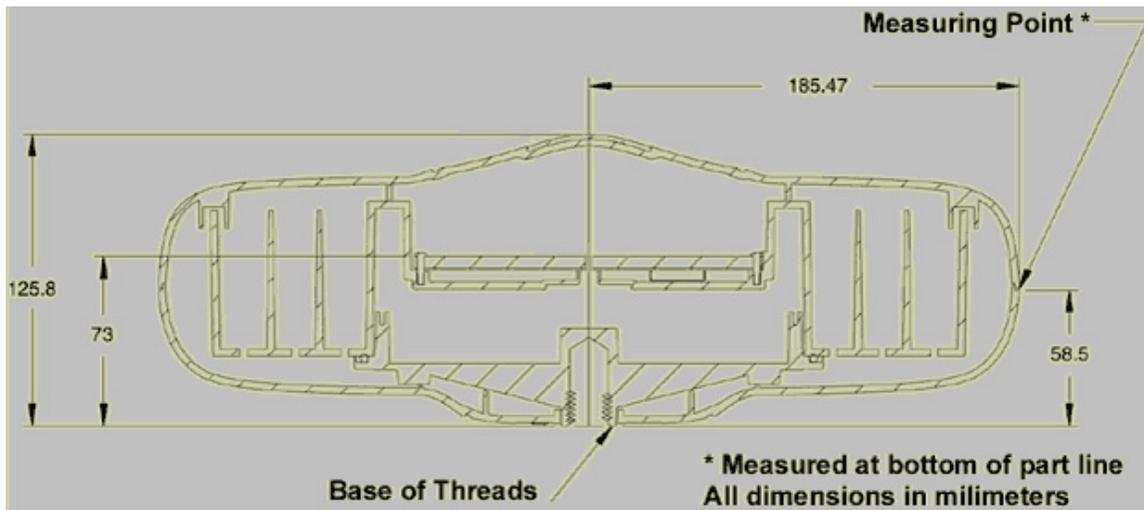
**Figure 7.** Antenna cross-section.
