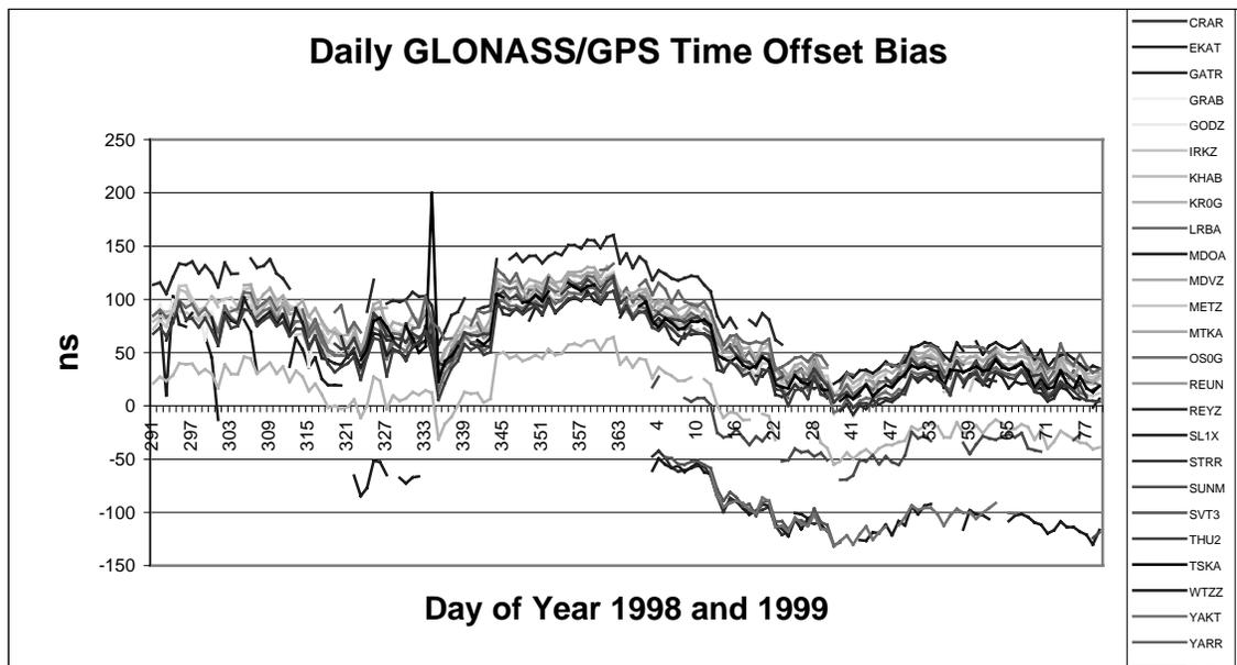
**Figure 3.** Daily GLONASS/GPS time offset bias for GPS weeks 980 through 1001. Only sites using Legacy or Z18 receivers are shown.
