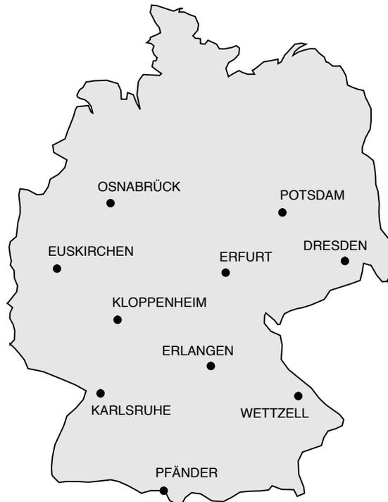
Figure 7: Planned GPS permanent network densification for Germany
