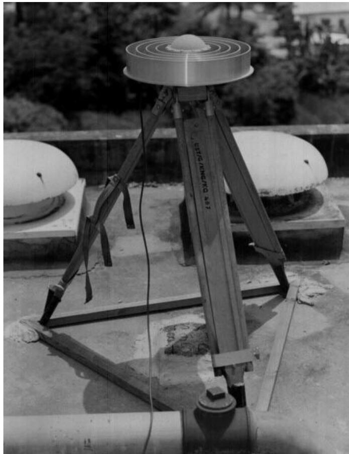
Figure 2: GPS antenna on top of the architecture building at UST
