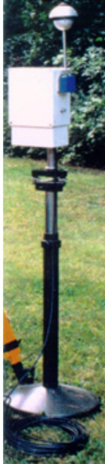
Figure 2: Meteorological sensor TM200
