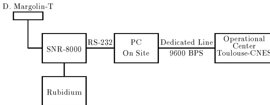
Figure 2: GPS System Configuration — Hartebeesthoek
