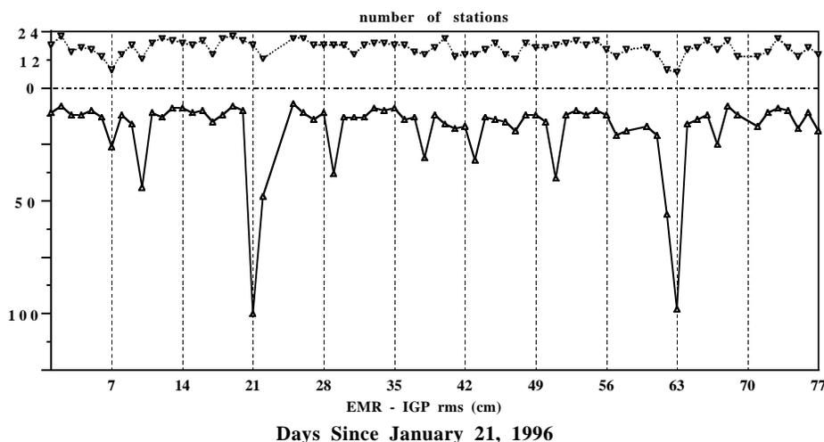
Figure 3: Number of stations (upper part) used for NRCan preliminary orbit computations and corresponding rms (lower part) of the differences between the NRCan preliminary orbits and the IGS combined preliminary orbits (IGP).
