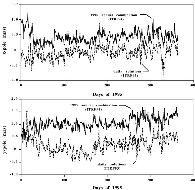
Figure 1: Differences between the EMR 95P01 and 96P02 EOP solutions and the IGS 95P01 EOP solution; (a) pole x-coordinate difference and (b) pole y-coordinate difference.
