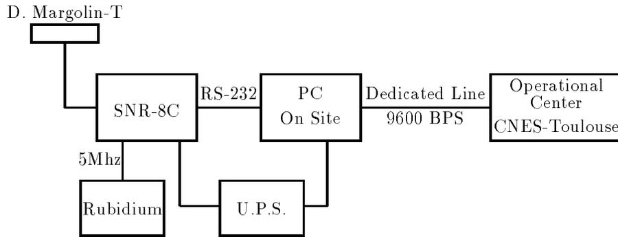
Figure 3: GPS System Configuration — Kerguelen
