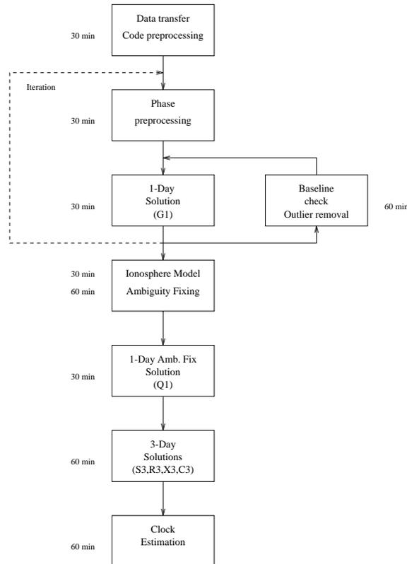
Figure 2: IGS Data Processing Flow at CODE (April 1996).
