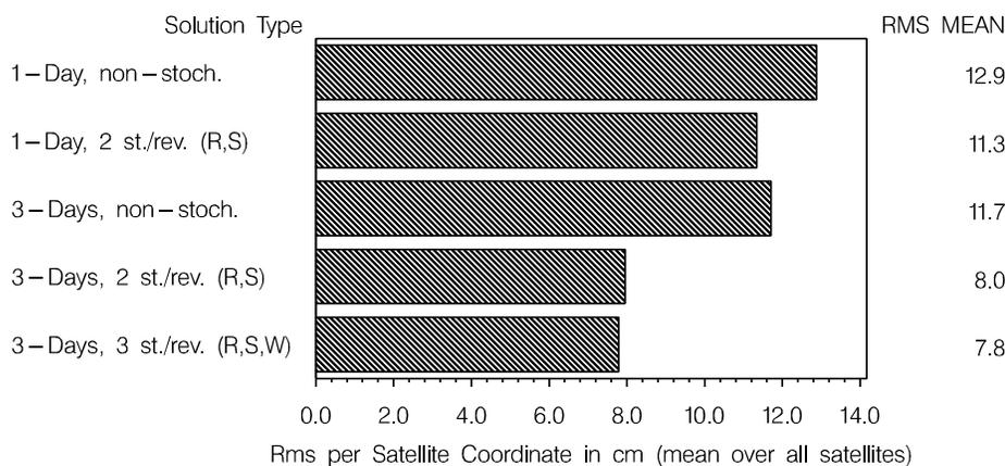
Figure 6: Comparison of orbit estimation strategies by fitting a 7-day arc through the 7 individual 1- or 3-day solutions of GPS Week 765 using the extended CODE orbit model.
