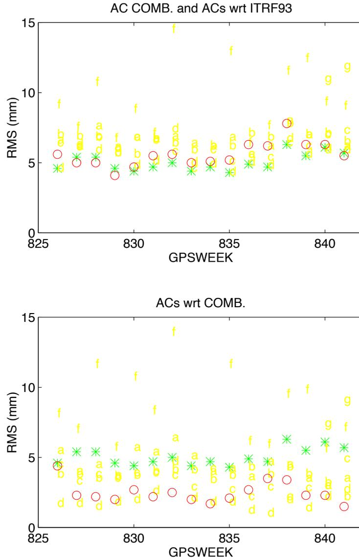
Figure 1: Comparison of SIO weekly SINEX with respect to ITRF93 and AC combined. The symbol '\*' denotes the rms series of AC combined, symbol 'o' denotes that of SIO. Letters are used for other centers.
