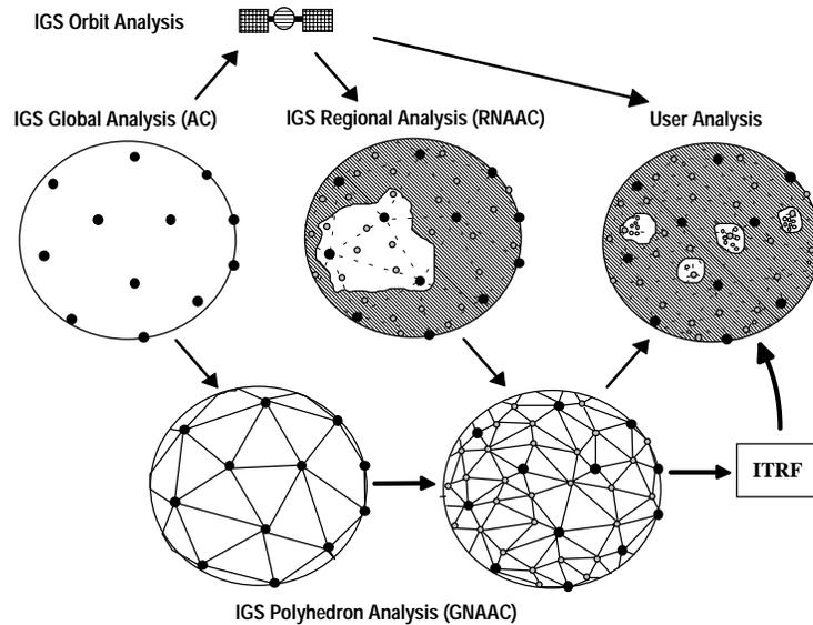
Figure 1: IGS Network densification by distributed processing
