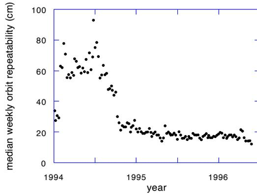
Figure 1: JPL orbit repeatability (3drms) since the official start of the IGS in 1994. Each weekly number indicates the median over all satellites and days during that week. (The daily number for a given satellite indicates the degree to which the precise orbit agrees with those of adjacent days near the midnight boundary.) Beginning in late 1994, the typical weekly value is about 20 cm or less.
