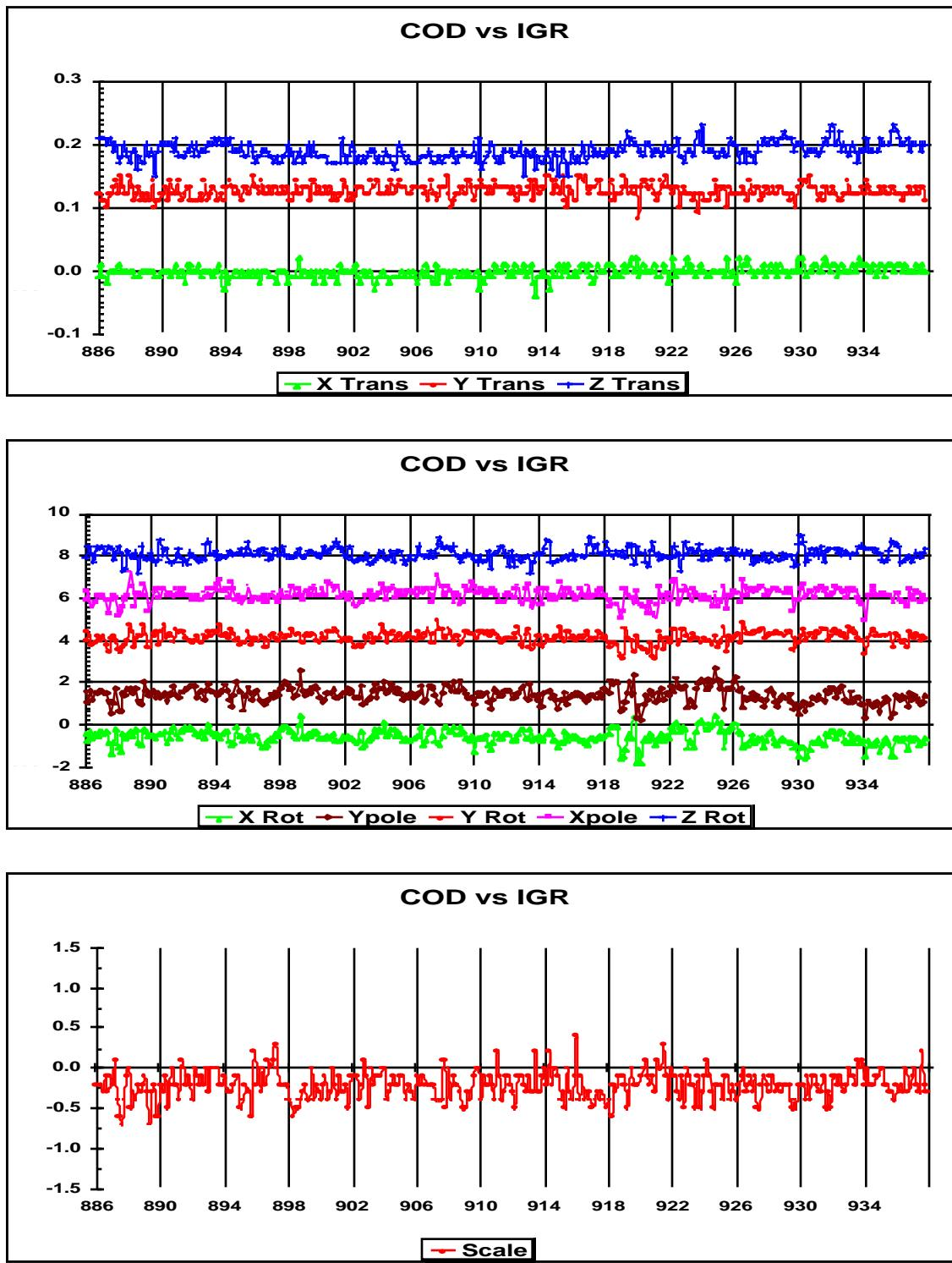
**Figure 10.** COD 1997: Rapid daily seven-parameter Helmert transformations (X, Y and Z Translations are each offset by 0.1 metre; X, Y, Z Rotations and Y and X pole differences are each offset by 2 mas)
