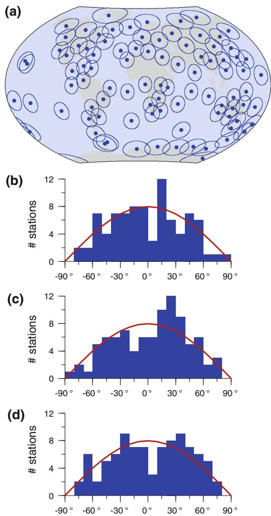
**Fig. 3** **a** Distribution of the 91 primary stations of the IGS08 core network. Each station is surrounded by a circle with a radius of 1,000 km. **b, c, d** Histograms of the corresponding  $(\phi_i^X, \phi_i^Y, \phi_i^Z)$  angles, respectively. The *red curves* represent the ideal cosine distributions of these angles
