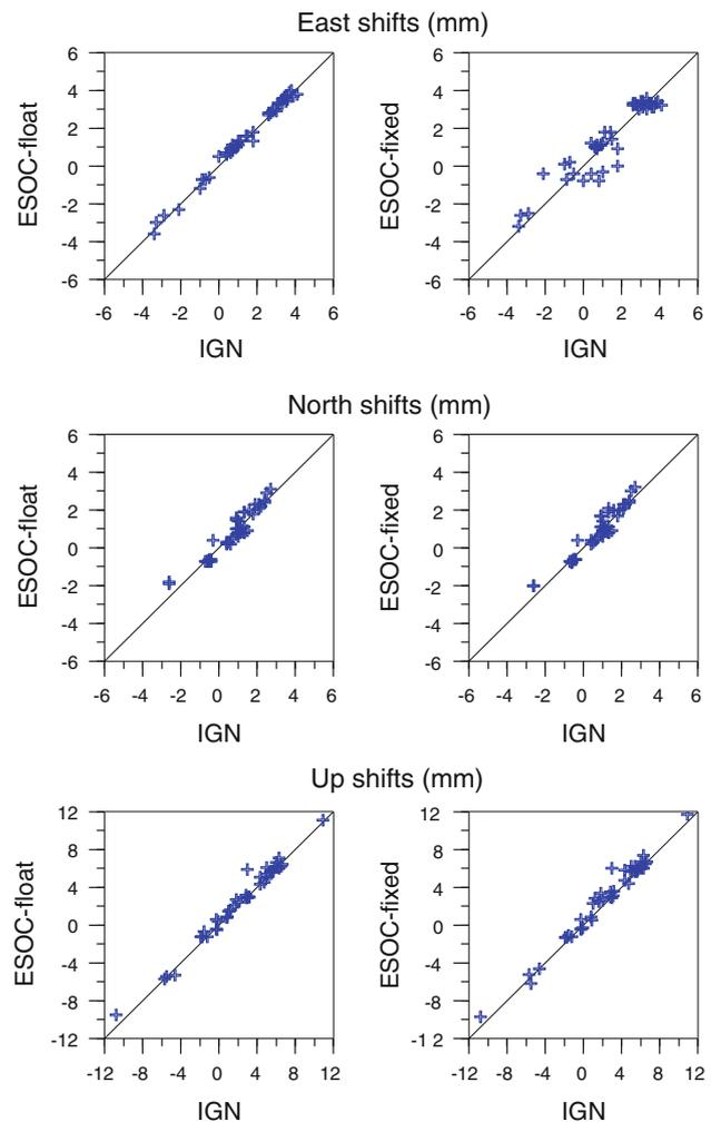
**Fig. 2** Comparison of the mean position shifts derived from the IGN and ESOC PPP tests
