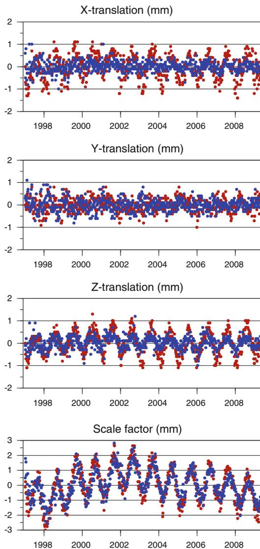
**Fig. 4** Translations and the change in scale estimated between the weekly synthetic solutions and ITRF2008. Parameters estimated with the full IGS08 network are shown by red dots, and those estimated with the IGS08 core network by blue dots
