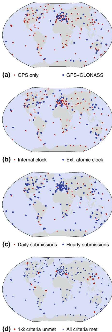
**Fig. 1** Distribution of IGS08 network stations **a** GLONASS-capable stations, **b** stations driven by external atomic clocks, **c** stations delivering hourly data, and **d** stations not fulfilling all criteria listed in Table 1
