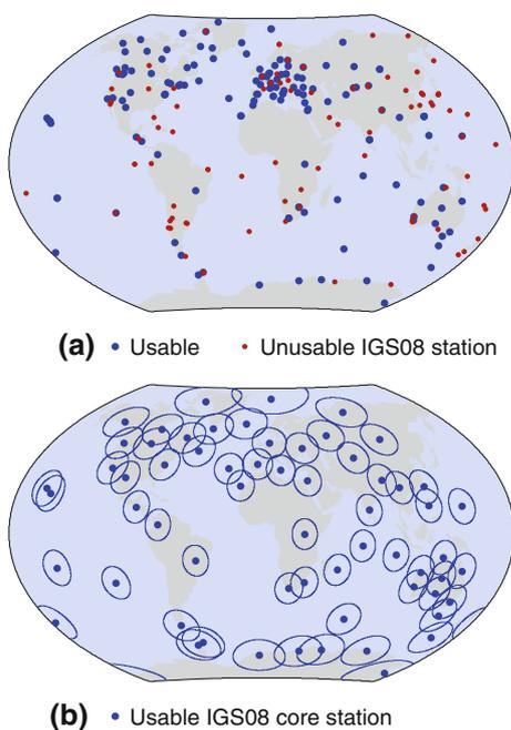
**Fig. 5** Distribution **a** of the 143 usable IGS08 reference stations in the IGS combined solution of GPS week 1638 and **b** of the 59 usable IGS08 core stations—including substitute stations—the same solution
