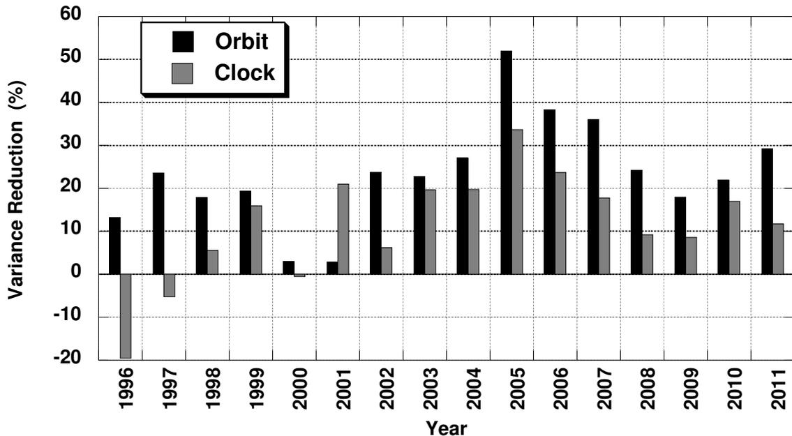
**Figure 1:** Variance reduction in orbit and clock precision of JPL’s first IGS08–based reanalysis of historical GPS data relative to our IGS05–based reanalysis. Precision is measured through the root–mean–square (RMS) of differences between neighboring daily 30–hour solutions during the overlapping 6–hour period. The average orbit and clock variance reduction for 1996–2011 is 25% and 12%, respectively.
