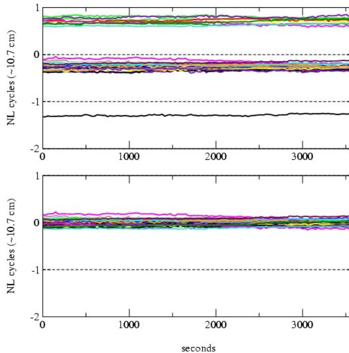
**Figure 5:** Example of the overlap differences between satellite clock estimates of day  $n+1$  (March 8, 2011) and day  $n$  (one curve per satellite). Before correction (top) and after corrections (bottom).
