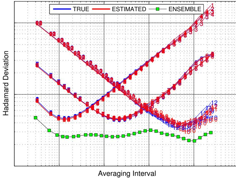
**Figure 3:** Timescale frequency stability results as measured by the Hadamard deviation statistic for a twelve clock simulation example based on three classes of clocks, where each class is differentiated by a relative different level of RWPH and RWFR noise.
