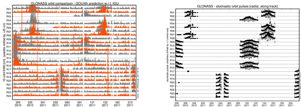
**Figure 2:** Quality of GLONASS orbits w.r.t. IGS finals (left) and estimated radial (grey) and along-track (black) stochastic pulses for eclipsing GLONASS satellites (right)
