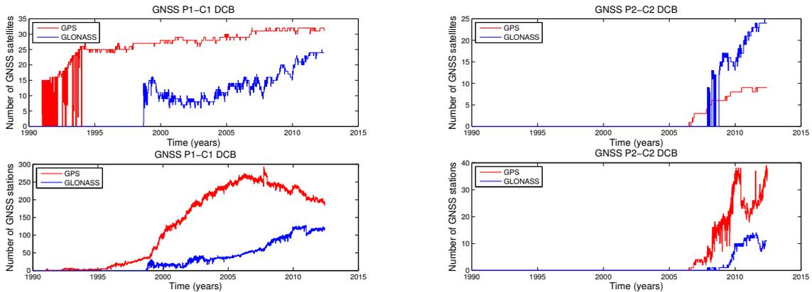
**Figure 7:** Time evolution of contributing number of GPS and GLONASS satellites (top) and corresponding receiver components (bottom), for P1–C1 (left) and P2–C2 (right) GNSS DCB reprocessing, carried out at CODE on the basis of 1990–2011 RINEX data.
