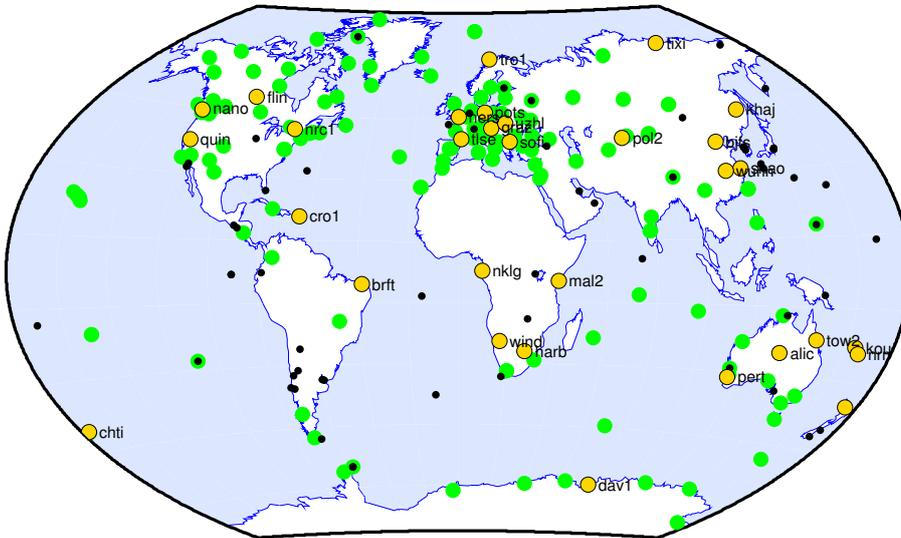
**Figure 4:** State map of the IGS08 network on GPS week 1674. Green dots are usable IGS08 stations. Orange dots are the 31 IGS08 stations which would be recovered with the adoption of IGb08. Black dots are unrecoverable IGS08 stations.
