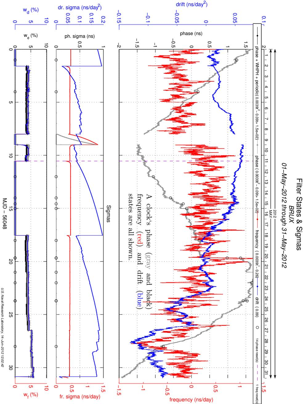
**Figure 9:** Sample plotting output of the v2.0 timescale filter states/sigmas for the IGS site BRUX. The plot shows the four base states, sigmas, and weights for the clock over a one month period. The black series correspond to the phase (including harmonics), the gray the phase without harmonics, the red series correspond to frequency and blue to drift. The legend also indicates any polynomials removed for plotting and/or phase or frequency breaks detected.
