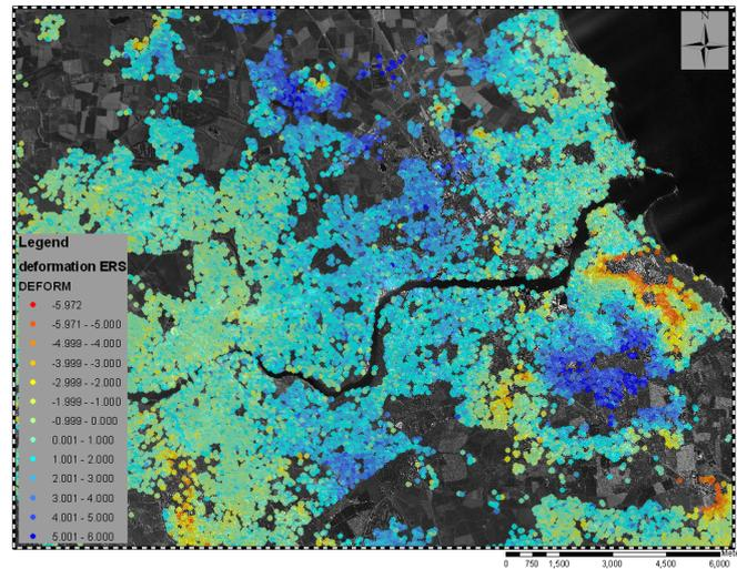
**Figure 6:** ENVISAT ASAR result for North Shields (2003–2008). TG site with GPS station are depicted as pink dot. Clearly visible are the various areas of relative land uplift and subsidence with respect to the reference scatterer (not shown). The VLM in the region around the TG are shown to be consistently between  $-2$  and  $+2$  mm/year (yellow to turquoise).
