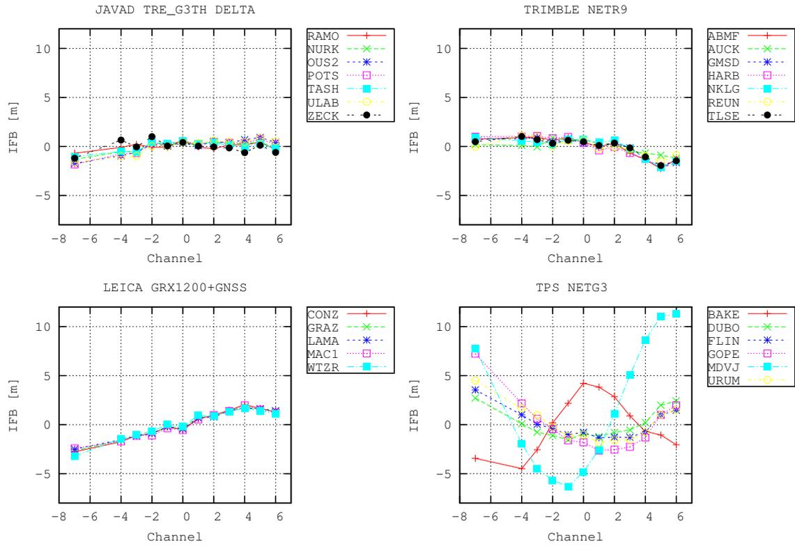
**Figure 3:** Inter-Frequency Code Biases per receiver type (mean values subtracted).
