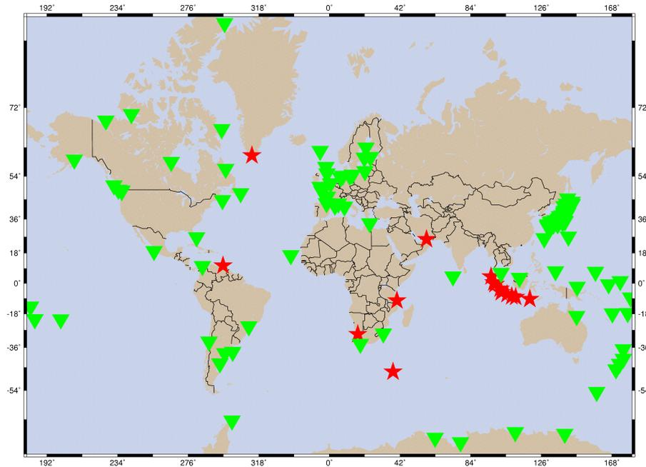
**Figure 1:** Current TIGA Network. Only stations are accepted as TIGA where, tide gauge, GNSS and leveling data is made public. (green triangles: TIGA Observing Stations, red stars: pending station approval)
