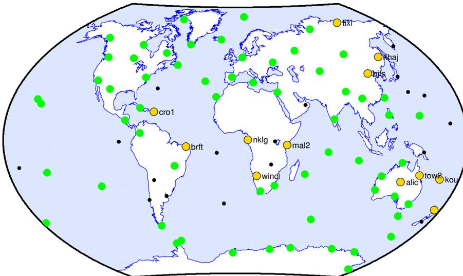
**Figure 5:** State map of the IGS08 core network on GPS week 1674. Green dots are usable IGS08 core stations. Orange dots are those which would be recovered with the adoption of IGb08. Black dots are unrecoverable IGS08 core stations.
