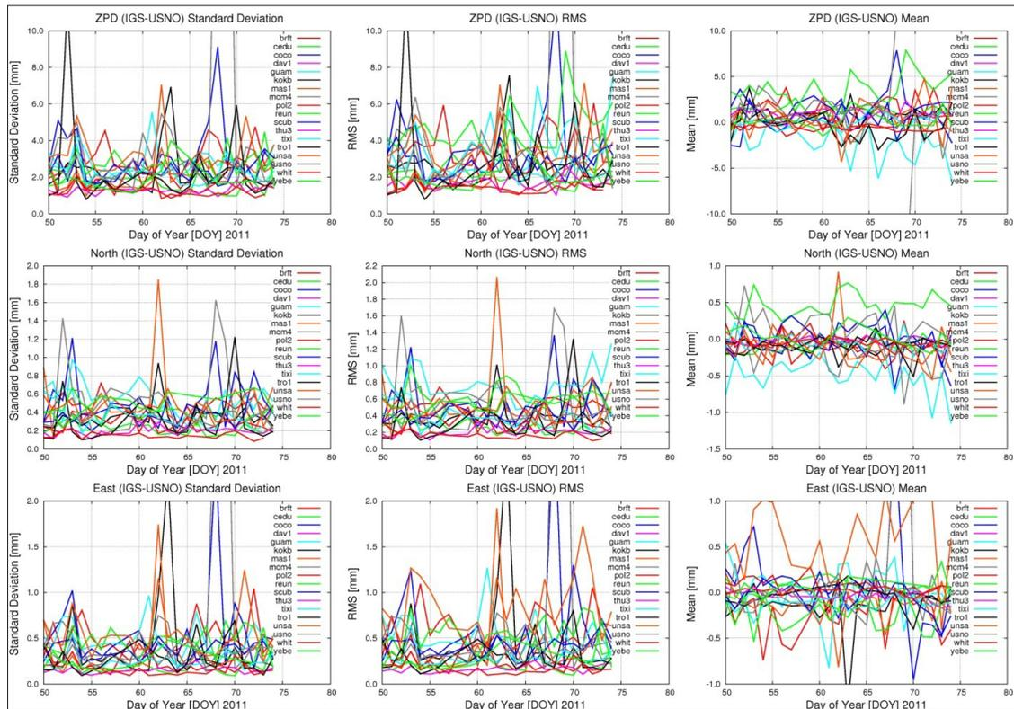
**Figure 1:** Comparison of USNO test troposphere solutions to existing IGS Final Troposphere estimates, in preparation for operational transition to USNO. ZPD = total zenith troposphere delay. Days of year 50–74 (28 Feb–14 Mar) 2011. From Byram et al. (2011).
