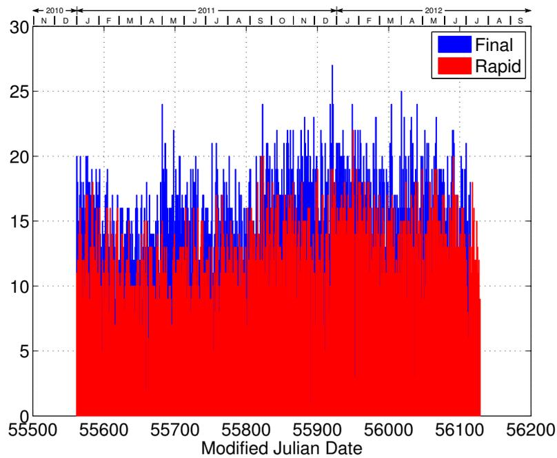
**Figure 6:** Histogram of the daily number of clocks in the IGS Final and Rapid timescale filters having phase estimate stabilities better than  $3 \cdot 10^{-15}$  at  $\tau = 21,600$  s as measured by the Hadamard deviation statistic.
