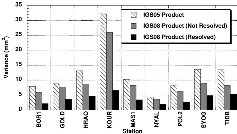
**Figure 2:** Impact of JPL’s orbit and clock product improvements (IGS05– to IGS08–based products), and single receiver ambiguity resolution (using WLPB product), on east component of station repeatability for 9 globally distributed stations with occupation histories of at least 12 years. Station repeatability is based upon daily static point positioning and with respect to velocity model for each station.
