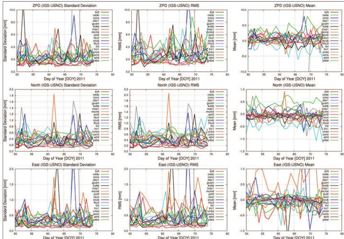
**Figure 5:** Comparison of USNO test troposphere solutions to existing IGS Final Troposphere estimates, in preparation for operational transition to USNO. ZPD = total zenith troposphere delay. Days of year 50–74 (28 Feb—14 Mar) 2011. From Byram et al. (2011).
