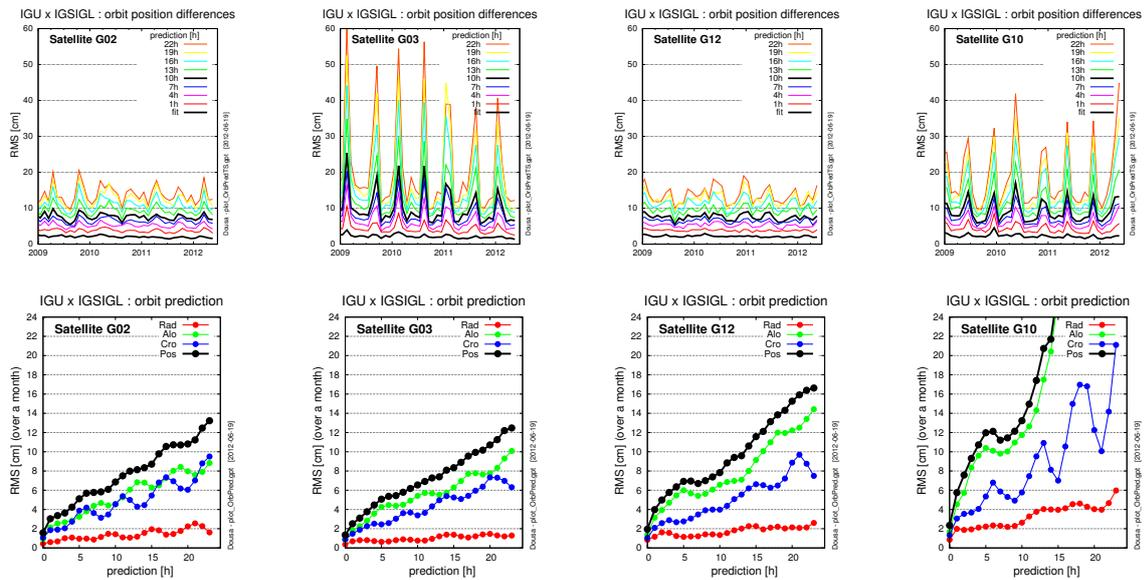
**Figure 3:** Plots show time-series of GPS satellite orbit quality (top) and the prediction of radial, along-track and cross-track monthly dependence on prediction (bottom). Two left plots show non-eclipsing and right eclipsing satellites. G02 and G12 are Block IIR, while G03 and G10 Block IIA satellites. Colors shows accuracy for fitted (0h) and predicted positions (1h, 4h, 7h, 10h, 13h, 16h, 19h, 22h) The orbits are compared to IGS finals
