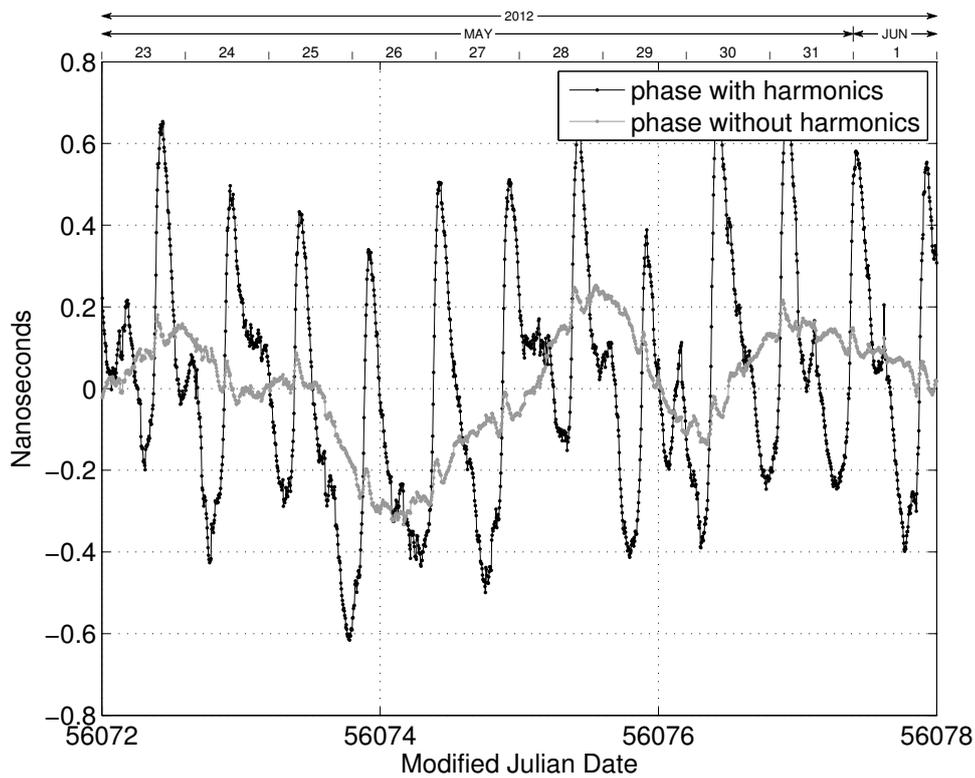
**Figure 8:** Timescale filter phase estimates of PRN 25 versus the IGS Final timescale IGST over the one week period 25 May through 31 May 2012. The black series shows the timescale phase state with harmonics while the gray series shows the phase minus the harmonics. An overall quadratic was removed from both series for plotting.
