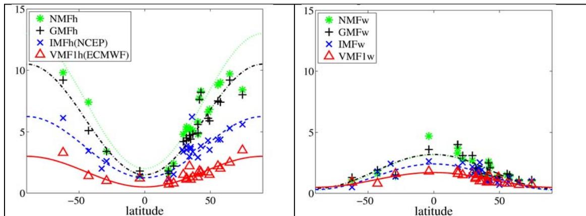
Figure 2 (from Niell (2006)). Standard deviation of station heights in mm from radiosonde comparisons in 1992 for the hydrostatic mapping functions (left plot) and the wet mapping functions (right plot). VMF1 has the smallest standard deviation, followed by IMF with a standard deviation that is about twice as large as that of VMF1. GMF is slightly better than NMF, but both empirical mapping functions cannot perform better since they contain only a seasonal term.
