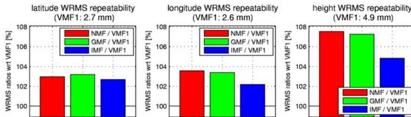
Figure 4 (from Tesmer et al. (2006)). Weighted RMS of VLBI station coordinates after removing the annual term for the latitude (left), longitude (middle), and height component (right). The repeatability with VMF1 is used as reference (horizontal line at 100%). The improvement in precision with VMF1 is about 3% for the horizontal components compared to NMF, GMF, and IMF, and about 7% and 5% for the height components.
