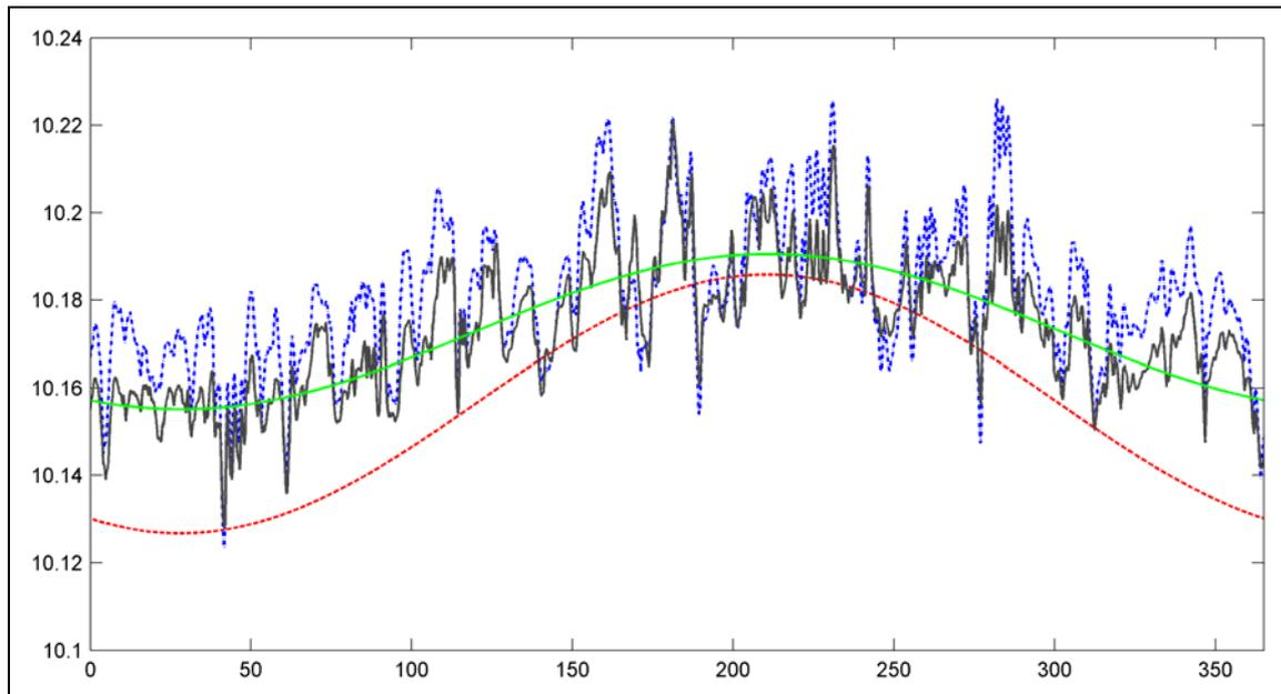
Figure 1. Hydrostatic mapping functions of NMF (red, dash-dash), IMF (blue, dash-dot), VMF1 (black, solid) and GMF (green, solid) at  $5^\circ$  elevation at station O'Higgins in the Antarctica during 2005. Especially around January, the NMFh is significantly smaller than the other mapping functions, which is the reason for lower station heights obtained with NMF at this station.
