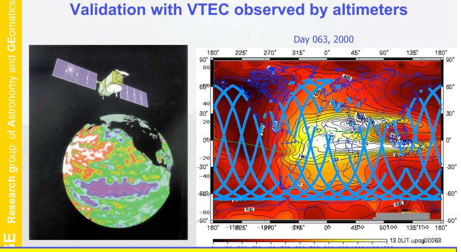
The direct VTEC measurements obtained from dual-frequency altimeters (TOPEX & JASON) over the oceans (typically far from GPS ground receivers) constitutes a good external data source of reference to characterize the iono maps accuracy in such "worst-case" scenario for GPS ionospheric maps.
