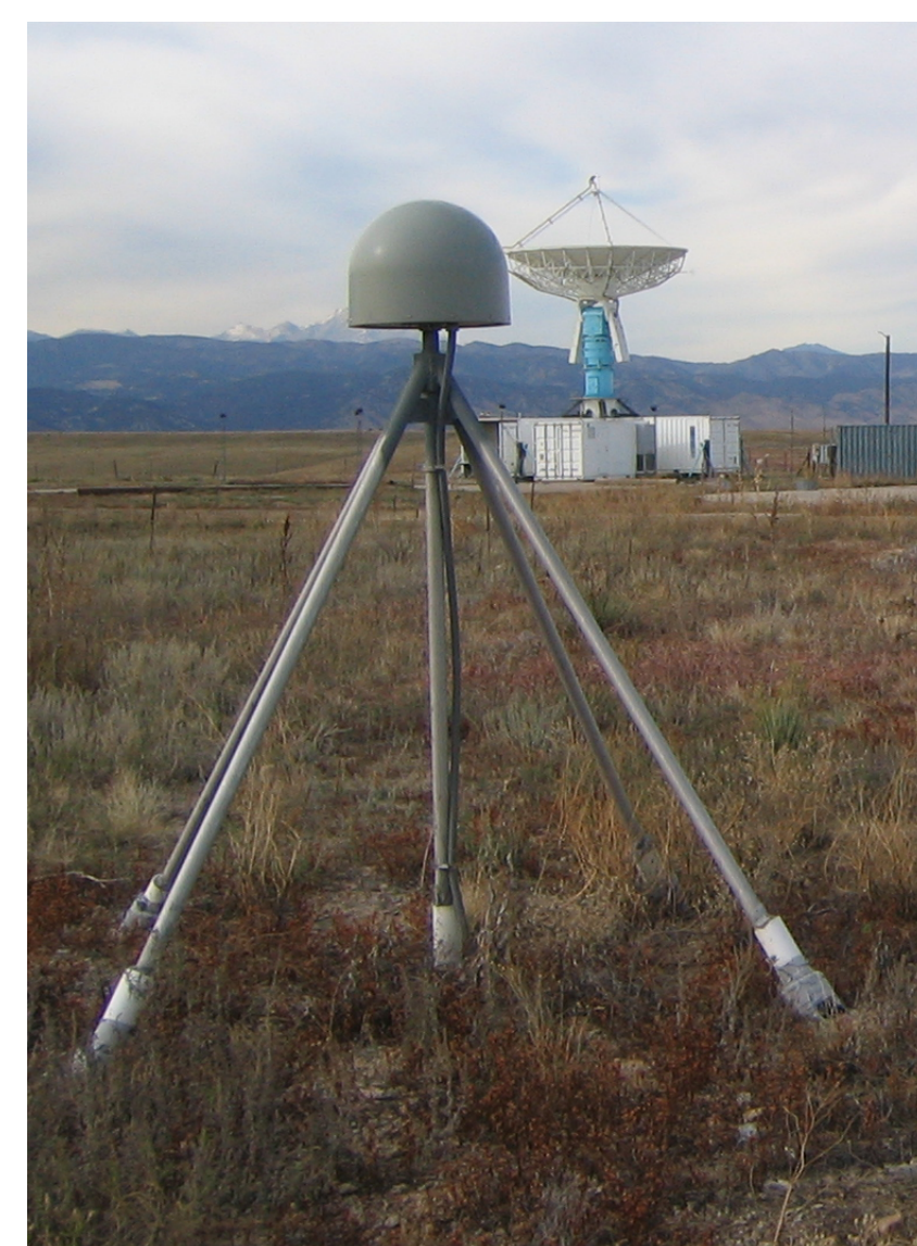
Deep drilled braced monument at Marshall field part of the Plate Boundary Observatory (PBO).
