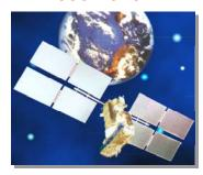
Developer NPO PM Flight Test phase Ordered 3 SV In orbit 1 SV To be ordered 9 Clock 1.10<sup>-13</sup> Life-time 7 years 2<sup>nd</sup> civil signal
