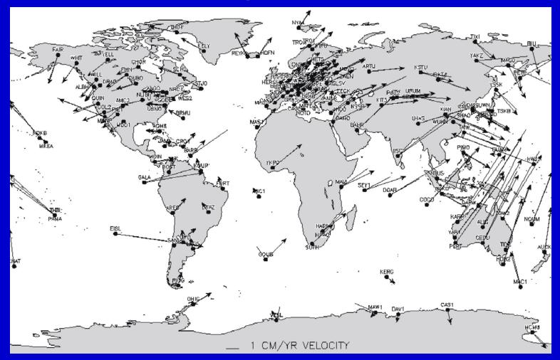
• The IGS monitors *plate tectonics* in "real time". Density of stations and time resolution of station motion are unprecedented.
