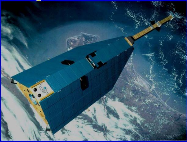
CHAMP, launched in summer 2000, explores gravity field (+magnetic field and atmosphere) using spaceborne GPS receiver.
