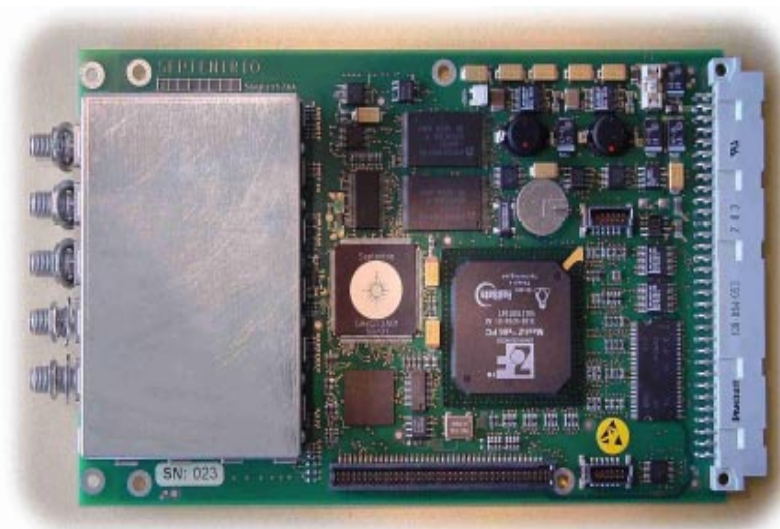
Figure 7. The outside view of PolaRx2, a Eurocard-formatted OEM board.
