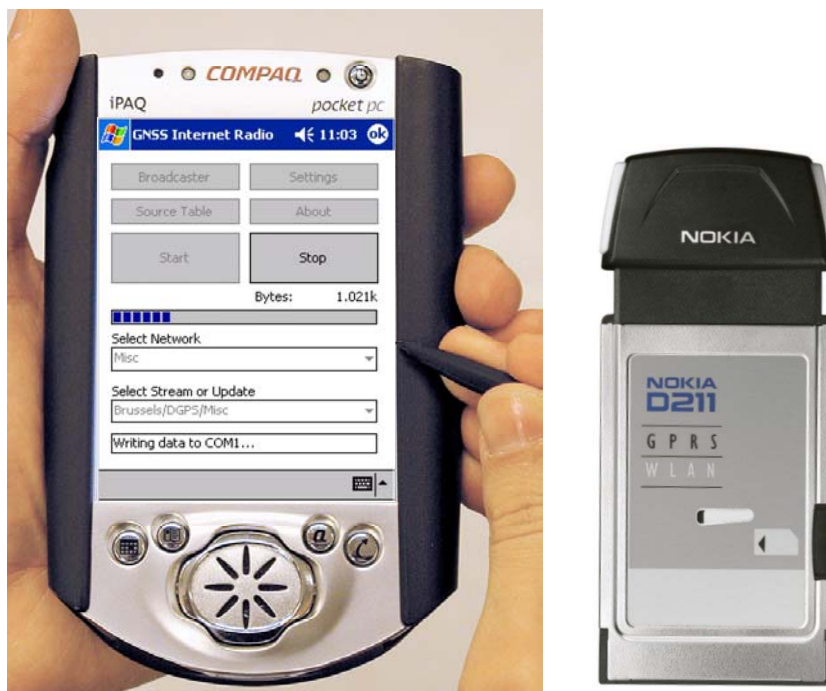
Fig. 3: Pocket PC with GNSS Internet Radio / GPRS modem
