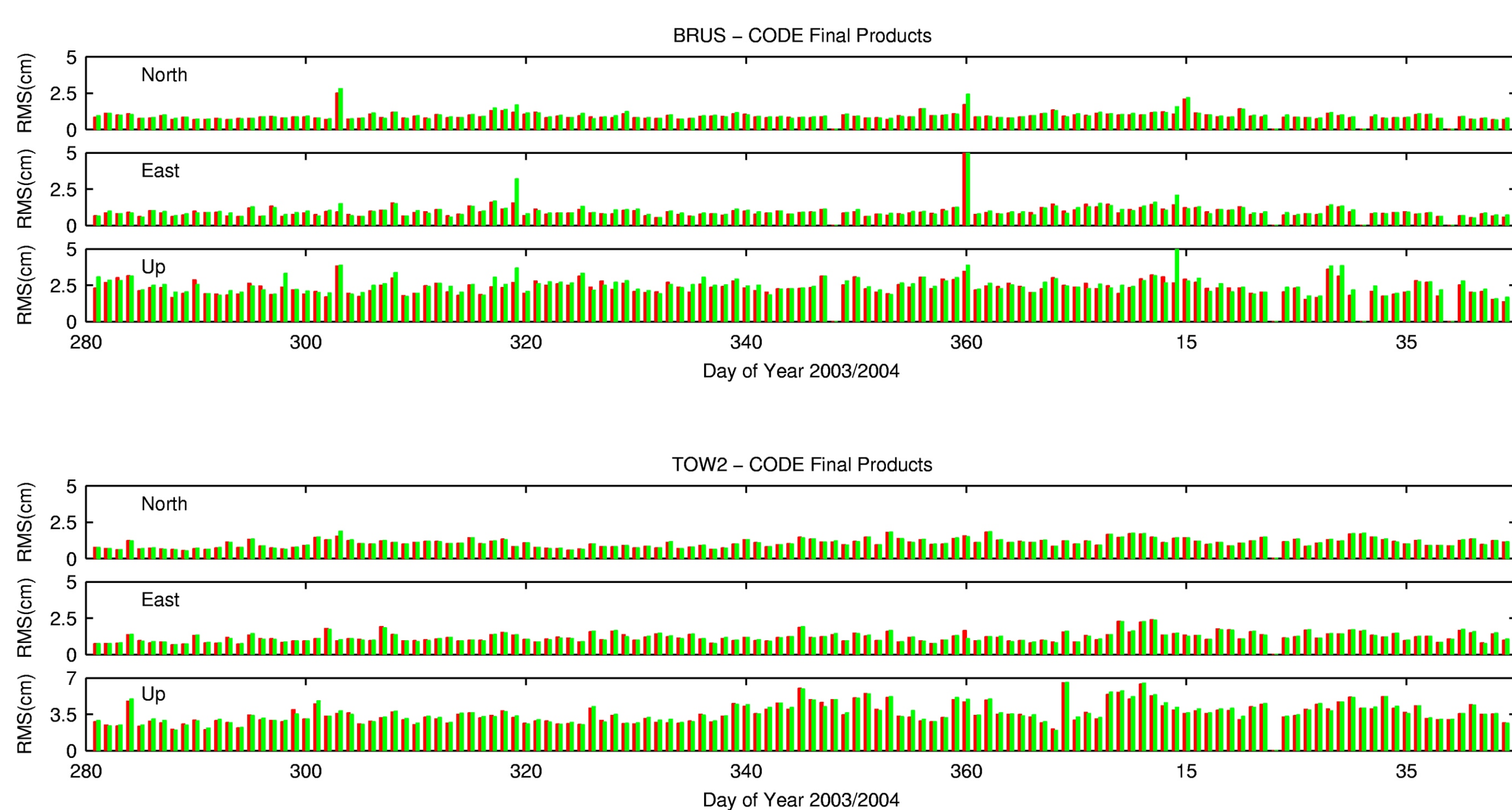
Figure 2: RMS errors (cm) per component of kinematic point positioning of BRUS and TOW2 using CODE final products, left bar: 30-second sampling (solution 1), right bar: official 5-minute sampling (solution 2).
