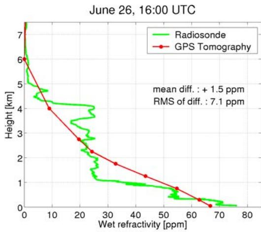
Fig. 5: Comparison of wet refractivity profiles derived from radiosonde observations and preliminary GPS Tomography results at station CINQ. The dots in the tomography profiles represent the layers of the voxel model.
