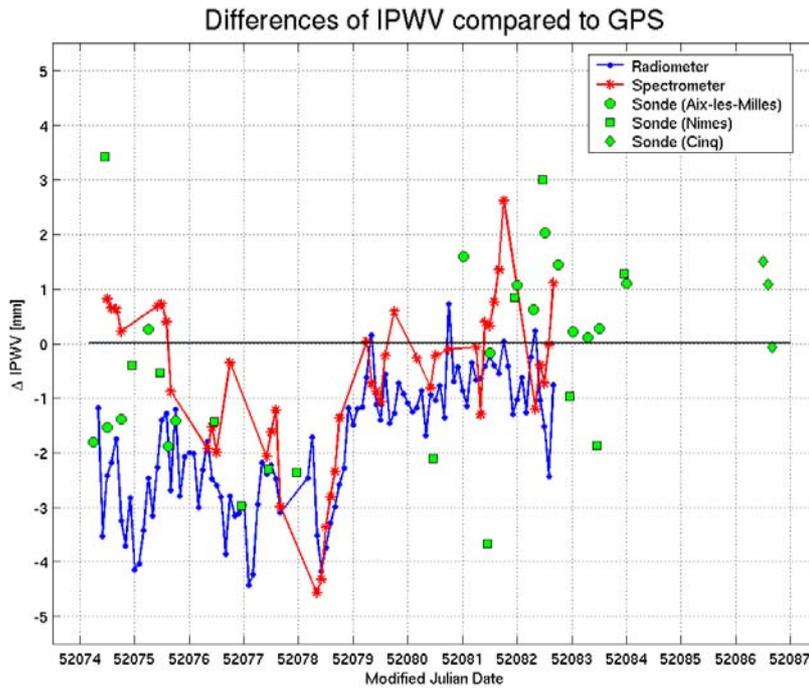
Fig. 3: Differences of IPWV. The reference is the GPS derived solution. A general overestimation of water vapor by GPS in the first half of the time span gets better in the second half.
