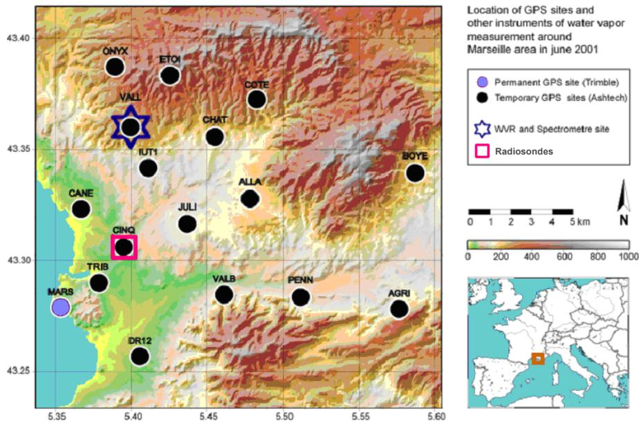
Fig. 1: GPS network and sites with further instrumentation in the ESCOMPTE campaign. Additional radiosondes were launched at Aix-les-Milles and Nimes (20 and 100 km to the Northwest). The height distribution of the GPS stations ranges between 33 m (station TRIB) and 586 m (station ETOI).
