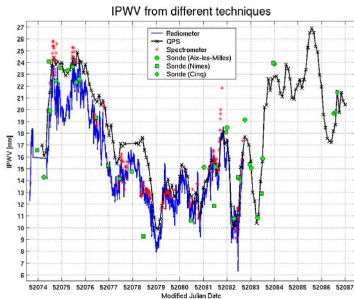
Fig. 2: Comparison of IPWV retrieved by different remote sensing instruments mounted at station VALL and additional data from several radiosondes nearby. The characteristic changes of the water vapor content above the station during the measurement period (14 to 27 June 2001) can be observed in the time series of the different measurement techniques.
