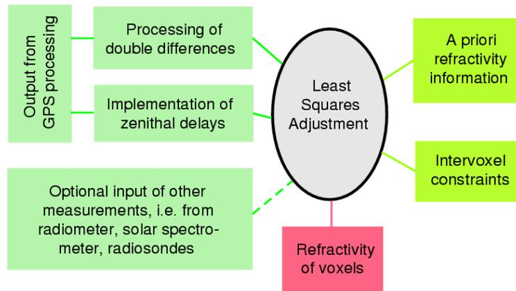
Fig. 4: Flow chart of the GPS Tomography software package AWATOS. The input data is shown on the left-hand side. On the right side, the possible introduction of additional pseudo-observations is outlined. They are necessary to get accurate and feasible results. Then, the refractivity can be calculated for each single voxel.
