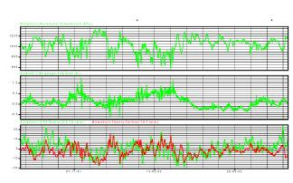
from tide gauge data. Loading calculations of the Baltic Sea show that 1 m of uniform layer of water corresponds 31 nm s<sup>-2</sup> in gravity and 10 mm in height. (Poutanen et al., (2004).
