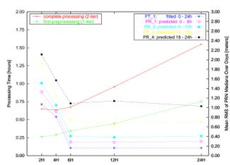
Fig. 2: The x-axis corresponds to the data pre-processing and NEQ lengths (variant ident.). The y-axis shows the processing time for two analysis steps. The y2-axis gives the mean RMS of the comparison of the resulting orbits with the IGS final orbits.
