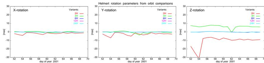
Fig. 4: Helmert rotations estimated from the comparison of five tested orbit solutions with respect to the IGS final orbits.
