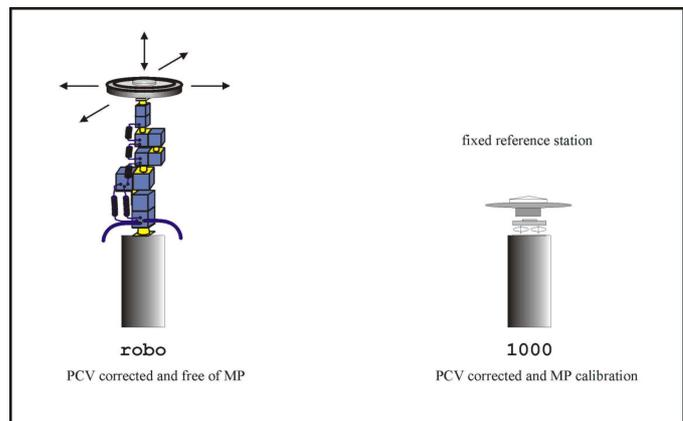
*moving antenna on robot (decorrelated MP) and static antenna (MP calibrated)*
