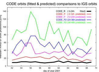
Fig. 11: The median RMS of CODE fitted and predicted orbits (CODE\_R, CODE\_P, CODE\_P2) characterizes the decrease of orbit accuracy when extending the prediction interval by a multiple of 12 hours.
