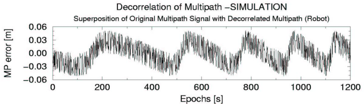
*simulation of observation difference between moving and static station*
