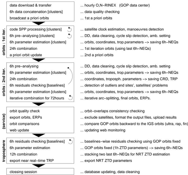
Fig. 2: The scheme of the GOP global NRT analysis for the orbit and tropospheric estimation.
