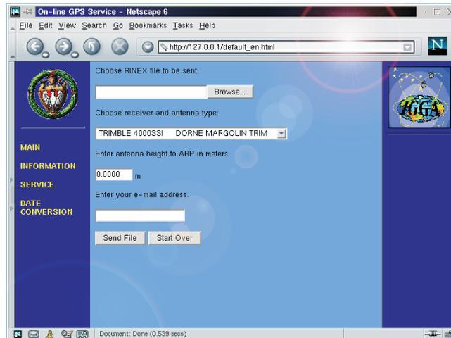
Appearance of the application form. User has to specify name of his (or her) RINEX file, type of the receiver and antenna, height of the antenna and e-mail address. The upload is performed using CGI script.
