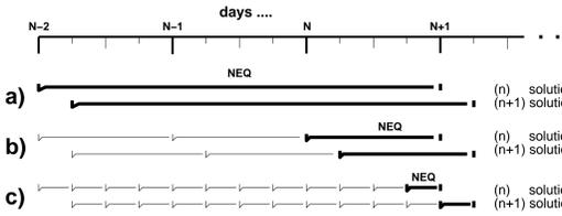
Fig. 1: The variants of a final 3-day solution generated using a different data pre-processing interval and NEQ combination technique (6-hours updating cycle): a) fully 3-day batch processing, no stacking, b) combined strategy, c) no-redundant pre-processing, fully stacking procedure.
