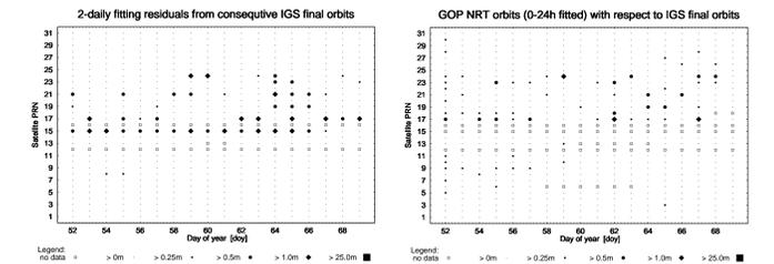
Fig. 5: Consistency of fitting two consecutive IGS final SP3 files with a single 2-day arc. Fig. 6: Comparison of fitted orbits (0-24h) for GOP NRT orbits.
