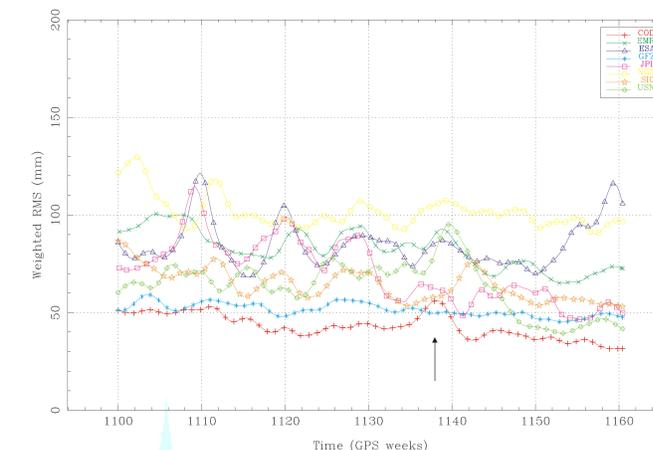
Figure 10: Smoothed weighted RMS for each AC rapid orbit solution with respect to IGS-combined orbit product
