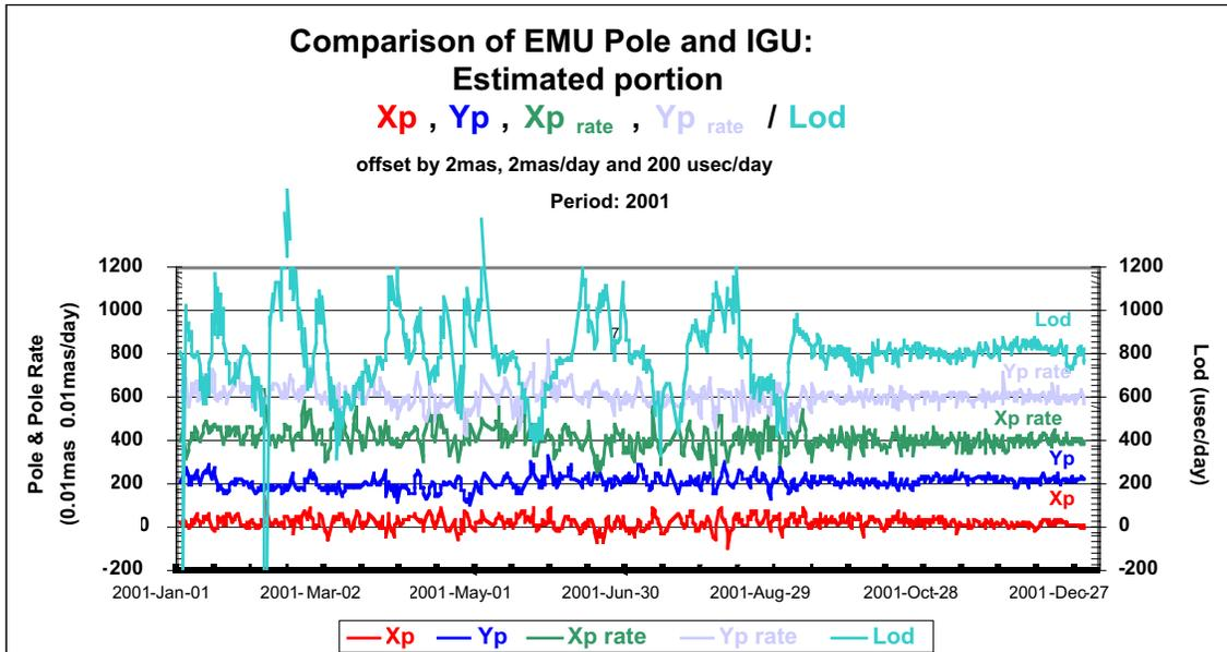
Figure 6: Comparison of EMU Estimated Pole and IGU for 2001:  $X_p$ ,  $Y_p$ ,  $X_{p \text{ rate}}$ ,  $Y_{p \text{ rate}}$  and  $Lod$ , each offset by 2 mas, 2 mas, 2 mas/day, 2 mas/day and 200 usec/day respectively.
