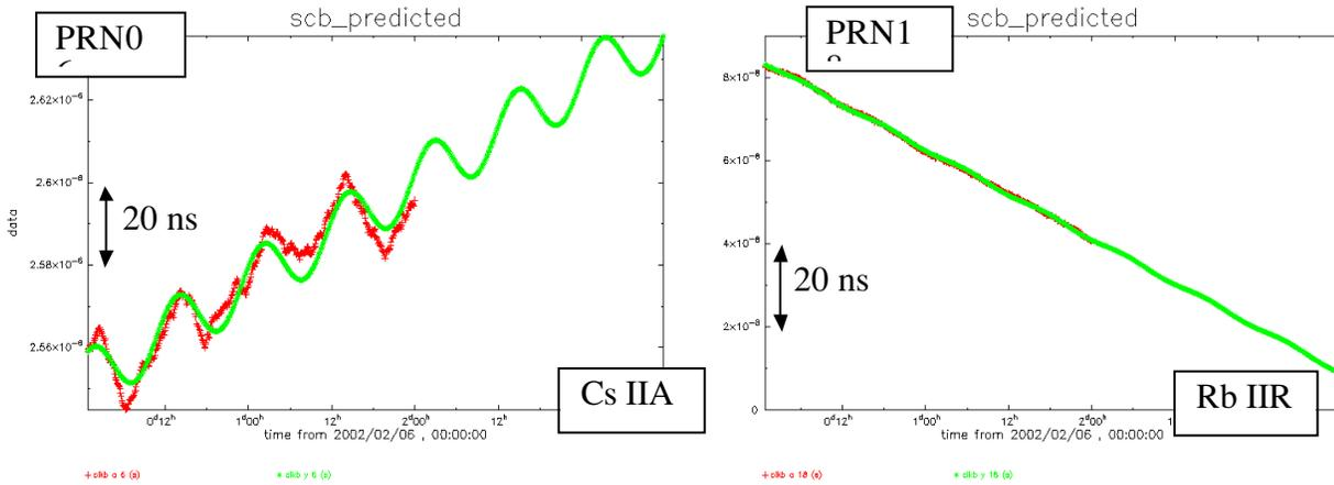
Fig. 3: Satellite clock biases estimated (red) and predicted (green) from 00:00 Feb 6<sup>th</sup>, 2002 (02037) (with the relativistic correction removed).
