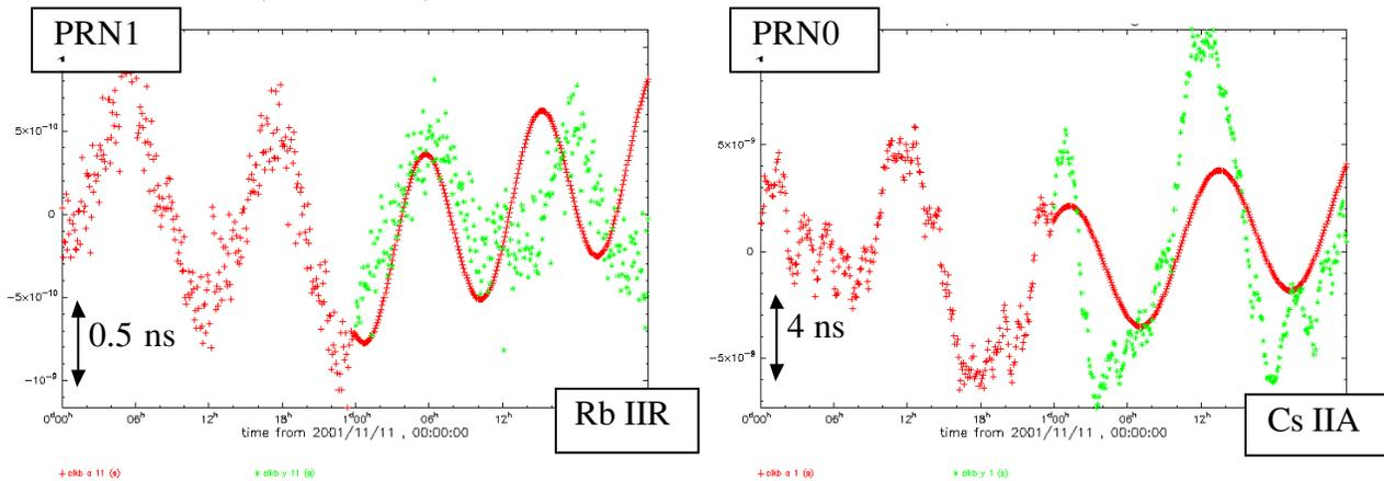
Fig. 6: Satellite clock bias values, submitted with the Ultra-Rapid (red) and estimated in the ESA Rapid process (green) for 48 hrs from 00:00 Nov. 11<sup>th</sup> 2001 (01315) (Offset and drift removed for plotting).
