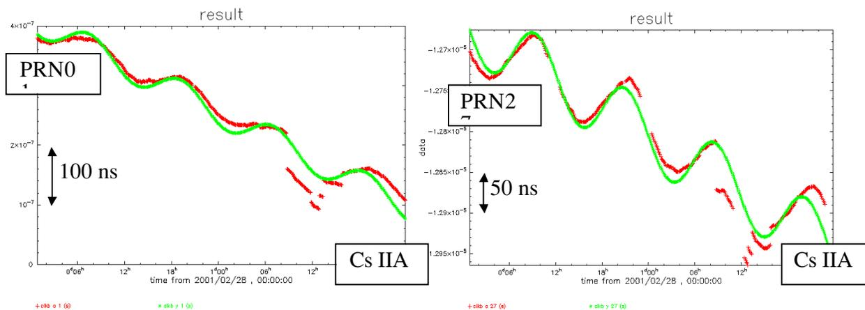
Fig. 2: Satellite clock biases estimated (red) and predicted (green) for 48 hrs from 00:00 Feb 28<sup>th</sup>,2001 (01059) (with the relativistic correction still included).
