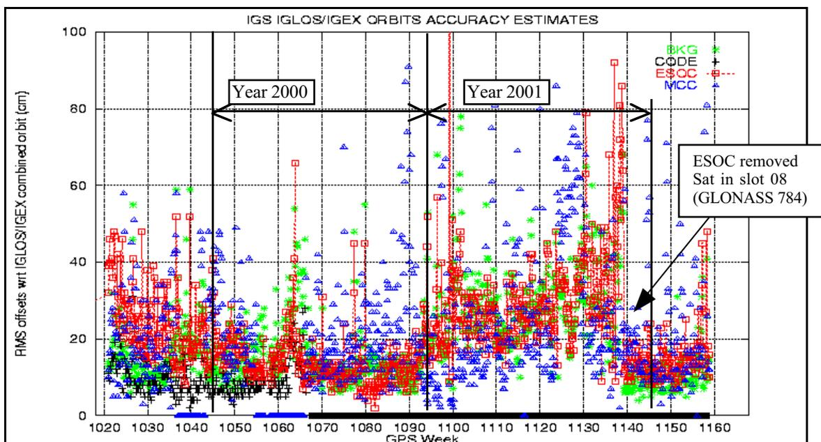
Fig. 9: IGLOS/IGEX AC orbit comparisons versus the combination.
