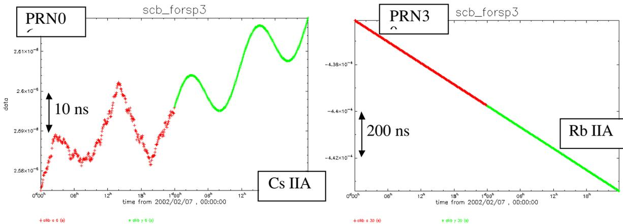
Fig. 4: Satellite clock biases estimated (red) and predicted (green) for 48 hrs from 00:00 Feb 7<sup>th</sup>, 2002 (02038) (with the relativistic correction removed).
