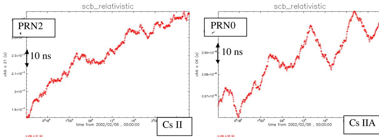
Fig. 1: Satellite clock biases estimated for 48 hrs from 12:00 Feb 6<sup>th</sup>,2002 (02037) (with the relativistic correction removed).
