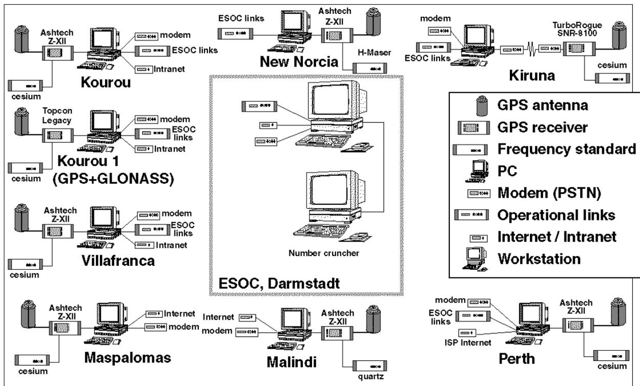
Figure 1: Configuration of the ESA stations by middle 2002.
