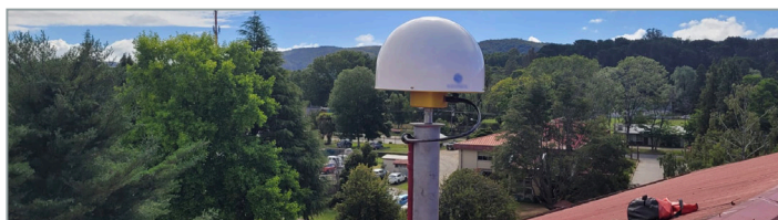
Figure 5: TEJA00CHL station, in process to include in IGS.
